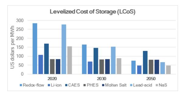
*Calculations of LCoS for seven storage technologies in Mexico when used for integration of solar PV.*
