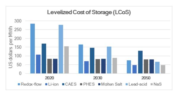
Calculations of LCoS for seven storage technologies in Mexico when used for integration of solar PV.
