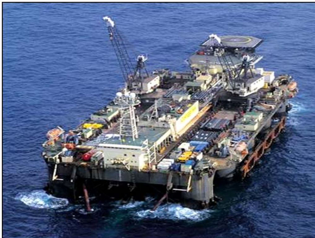
Figure 6-13 Castoro-Sei pipe-laying vessel.
