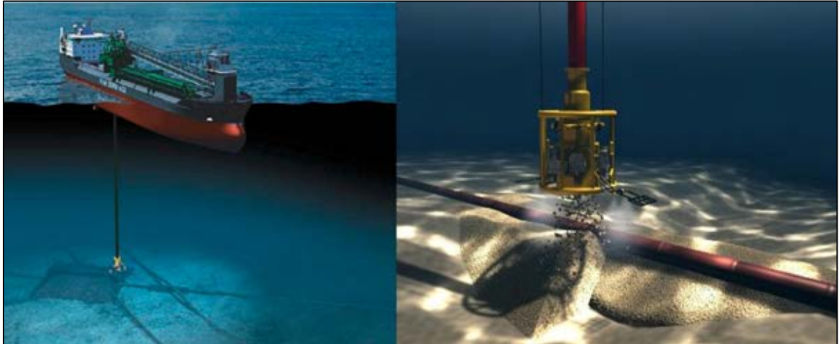
Figure 6-17 Rock placement on the seabed through a fall-pipe.
