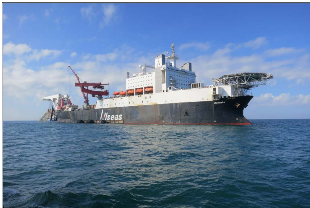
Figure 6-14 Typical DP vessel – Allseas Solitaire .
