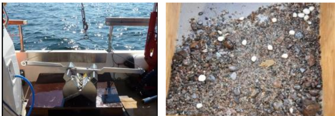
Figure 7-3 Sampling of infauna was undertaken with a Van Veen sampler (left). An example of an infauna sampling (right)
