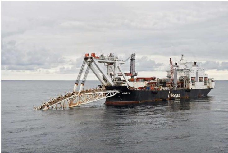
Figure B-1 Pipe-lay vessel in operation
