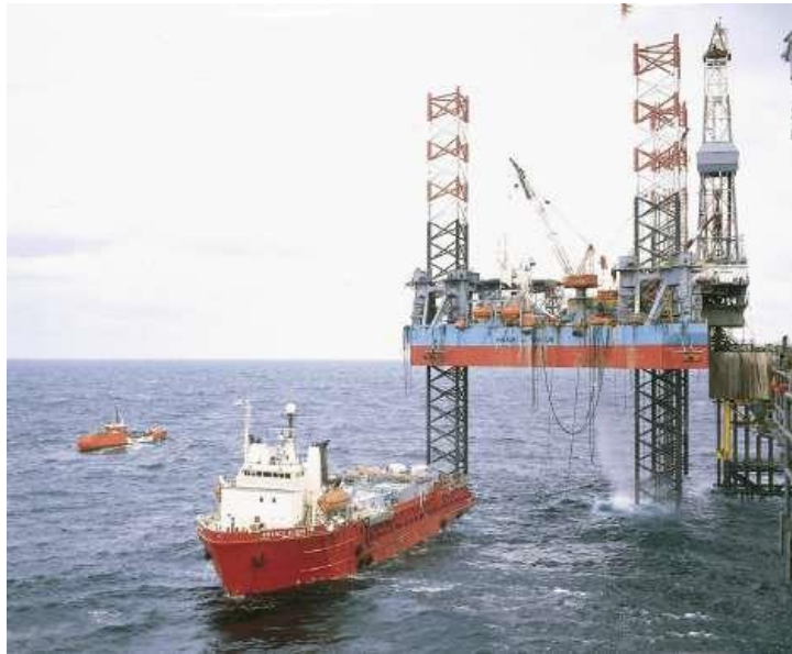
Figure E-1 Stimulation vessel ready to rig up for well stimulation
