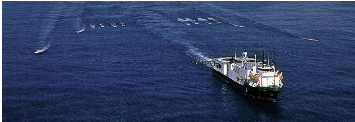
Figure A-2 3D seismic survey /6/
