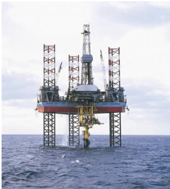
Figure D-1 Typical jack-up drilling rig (Maersk Endeavour), here situated at the Kraka STAR platform
