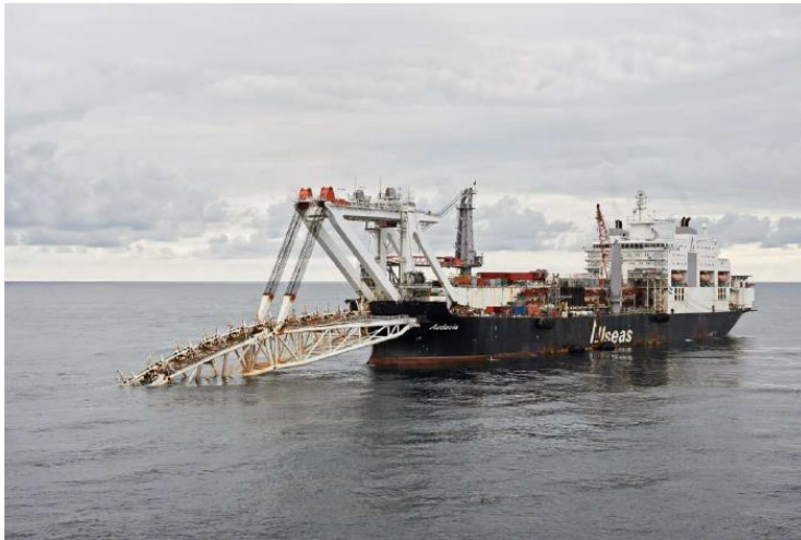
Figure B-1 Pipe-lay vessel in operation
