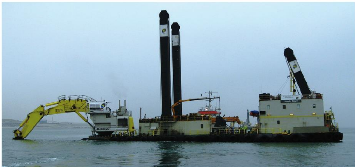
Figure 3-14 Typical backhoe dredge for trenching in shallow water.
