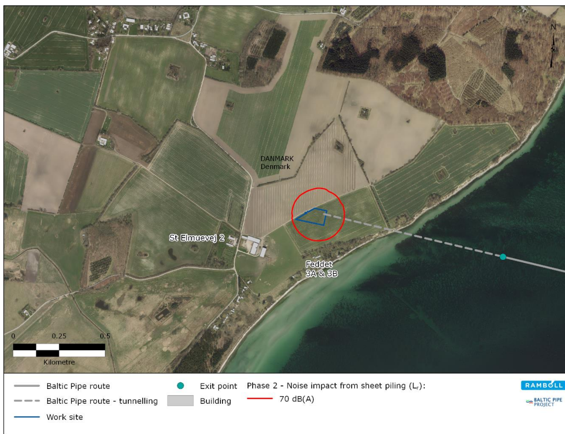
Figure 9-33 Noise map for phase 2, sheet piling and excavation (launch shaft) (1-2 weeks duration) presenting the noise contour for 70 dB(A) level. Sheet piling is expected to take place within regular working hours, where the applied guiding limit value is 70 dB(A). The 40 dB(A) noise contour is not presented, as it occurs primarily outside the extent of the map.
