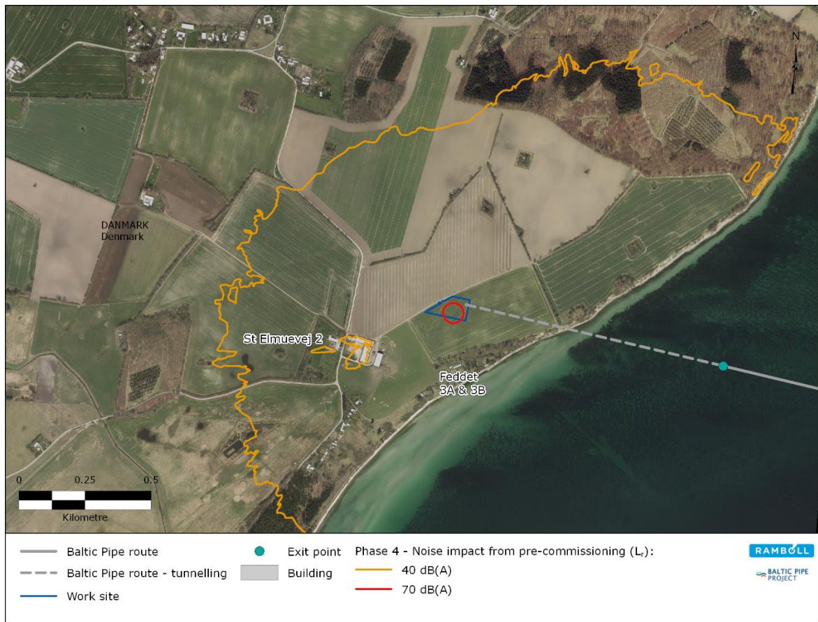
Figure 9-35 Noise map for phase 4, pre-commissioning (two months), presenting the noise contours for 40 dB(A) levels and 70 dB(A) levels. The activities during this phase will take place 24 hours a day.
