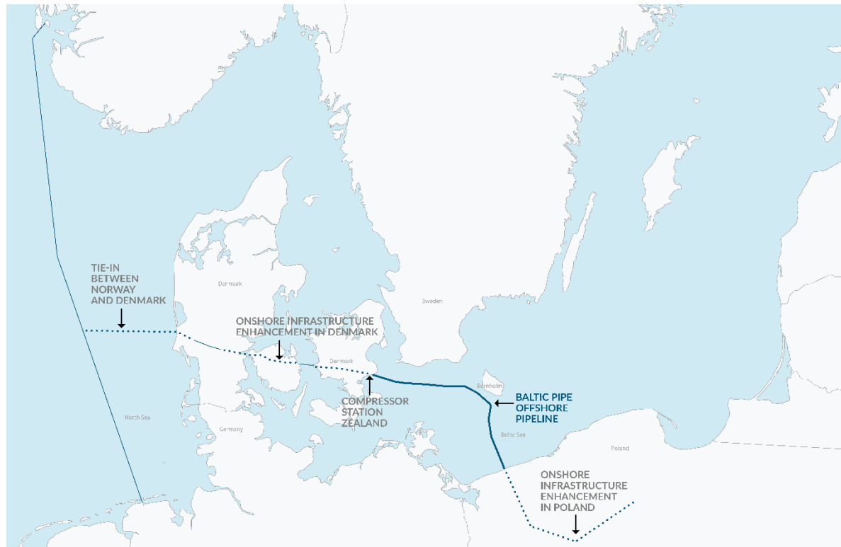
Figure 1-1 Schematic of the five major components of the Baltic Pipe project.
