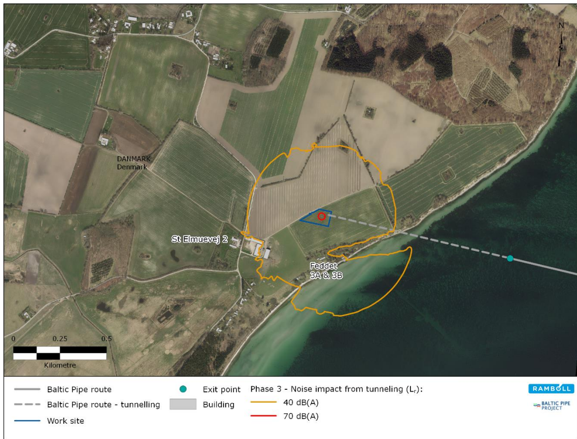
Figure 9-34 Noise map for phase 3, tunnelling (20 weeks duration), presenting the noise contours for 40 dB(A) levels and 70 dB(A) levels. The activities during this phase will take place 24 hours a day.
