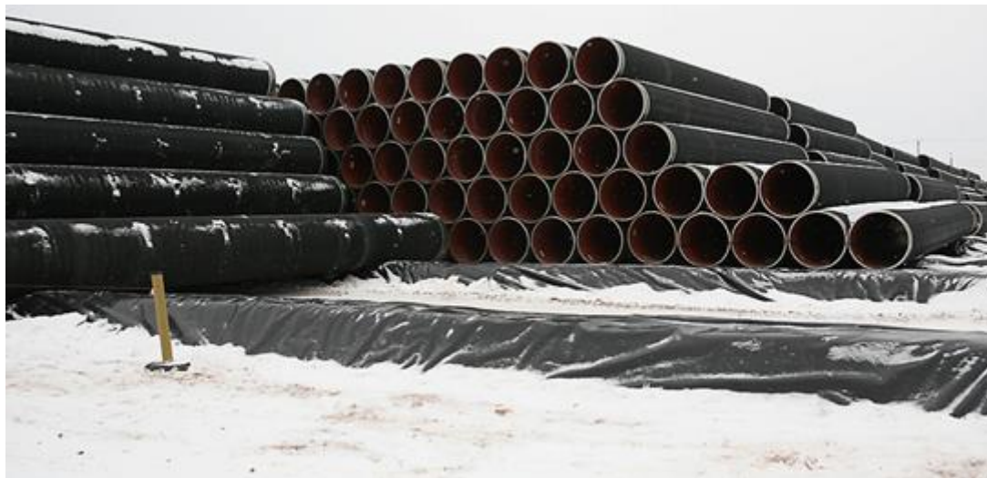
Figure 3-23 Example of storage of weight coated pipe joints in a port (Rambøll, 2018b).
