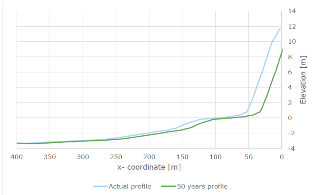
Figure 3-13 The actual cross-shore coast profile at Faxø South, shown together with the profile after 50 years, as calculated using geomorphological modelling (Rambøll, 2018e).
