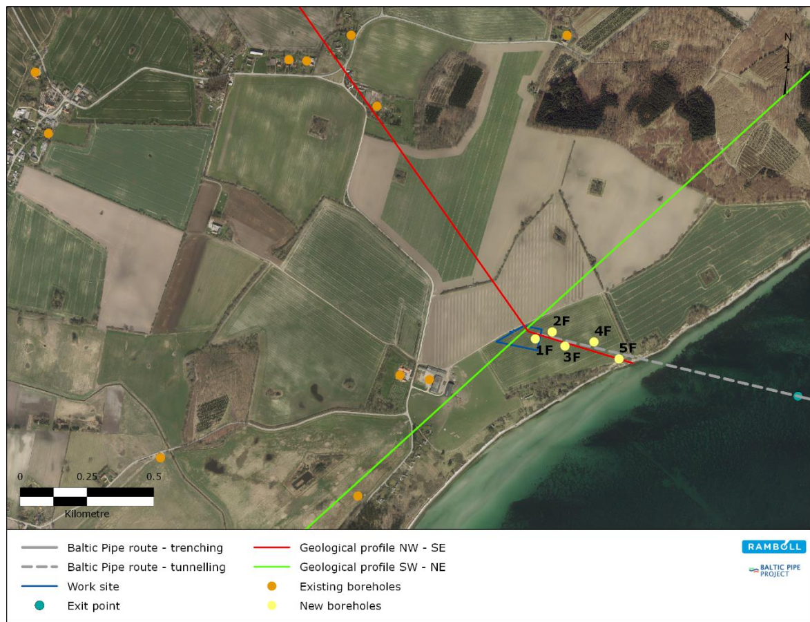
Figure 9-28 Location of boreholes and geological profiles.
