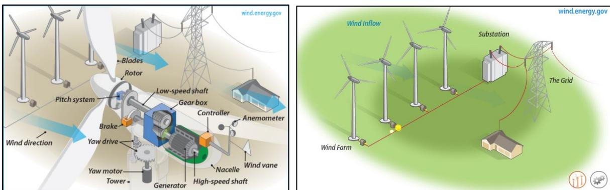
**Figure 11** General turbine technology and electrical system.
