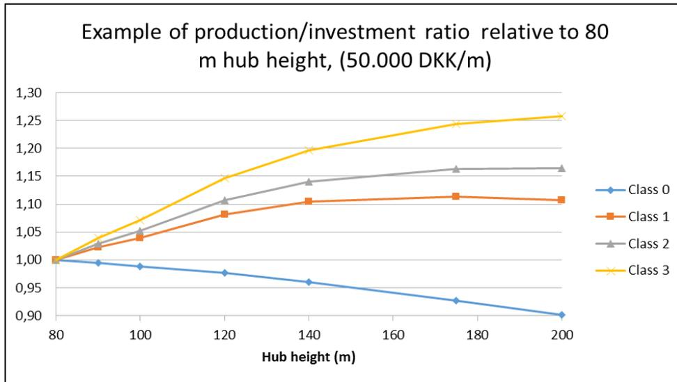
Figure 24 Similar, the production increase relative to the investment cost based on current available Vestas turbines, for increasing height, where costs are extrapolated using DKK 50.000 per m hub height increase, the rotor area is kept constant.
