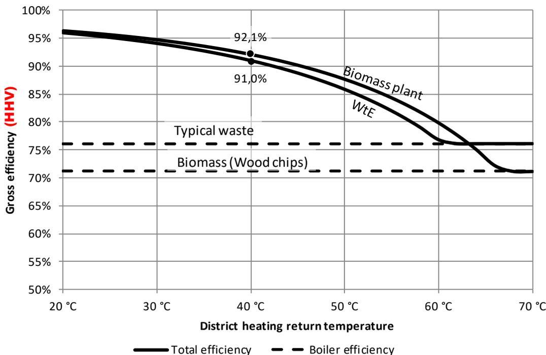
Figure 9. Total HHV-based efficiency estimate for WtE plants<sup>7</sup> and biomass plants<sup>8</sup> given varying DH return temperatures [5] – or temperature of the cold media of a heat pump.
