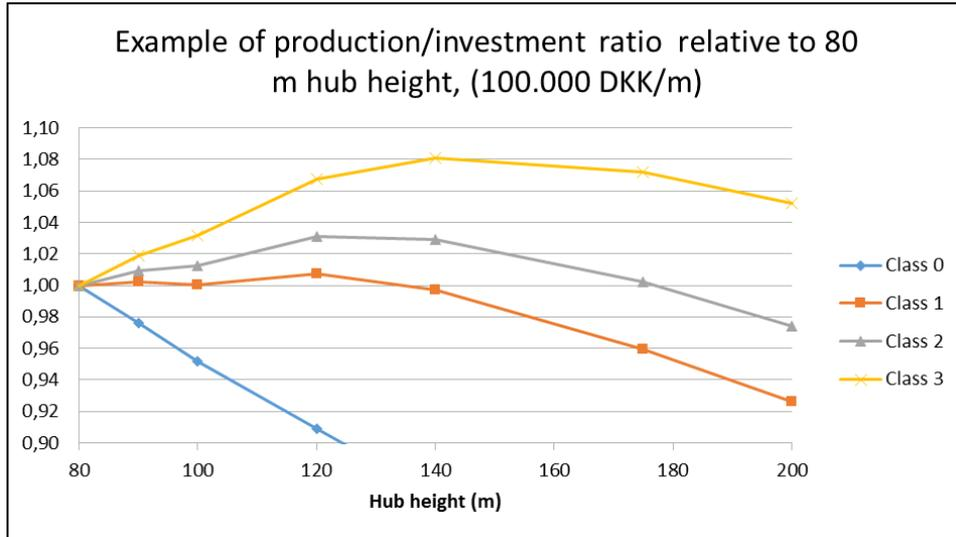
Figure 23 The production increase relative to the investment cost based on current available Vestas turbines. By increasing height, costs are extrapolated using DKK 100.000 per m hub height increase; the rotor area is kept constant.
