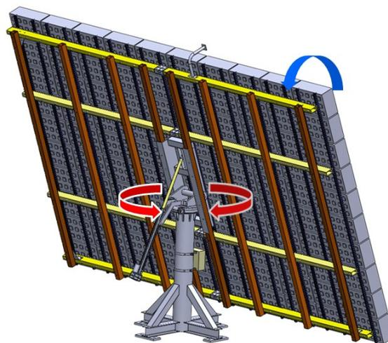
Figure 5 A generic dual axis PV system (Ref. 11)
