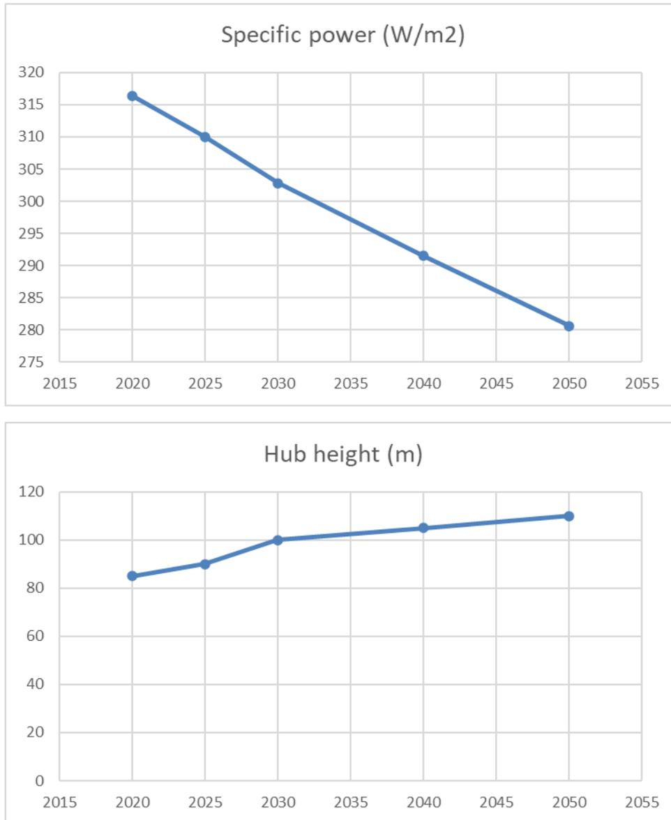
Figure 34 Expected development in production (full load hours (FLH)), specific power and hub height for on shore wind turbines located in DK.
