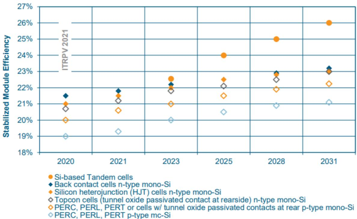
Figure 9 Efficiencies of different cell types (Ref. 9).
