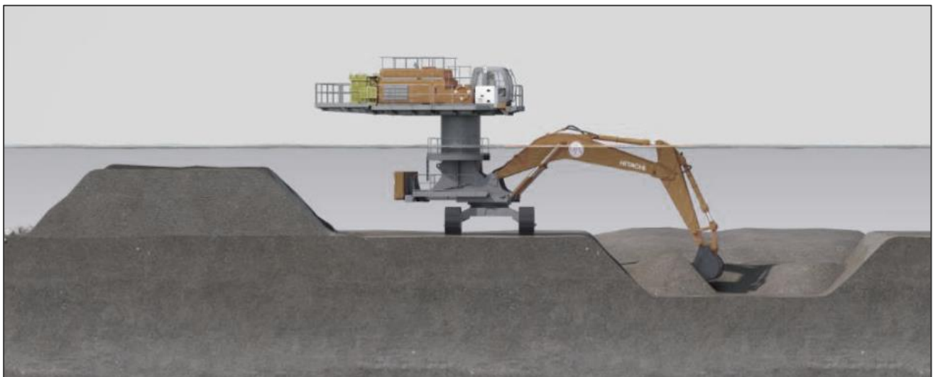
Figure 8.4: Illustration of a backhoe dredger excavating a trench in a nearshore setting. The excavated sediment is moved to one side of the cable trench to allow for natural backfilling. Illustration from Jan De Nul.
