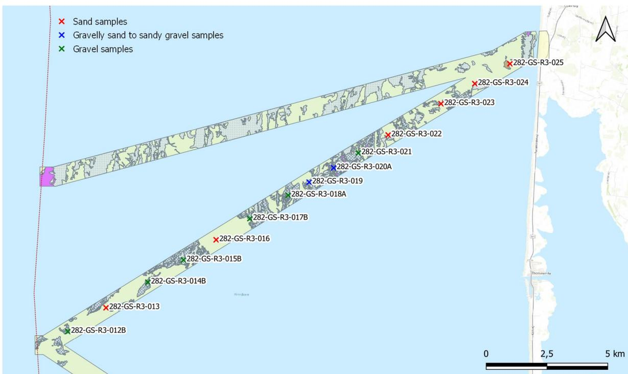
Figure 4.9: Grab samples used to calculate the average particle size distribution in the ECC area.
