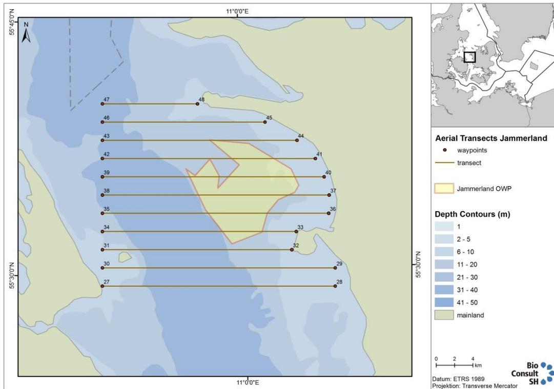
Figure 2.2 Aerial survey transect design for the Jammerland survey including the proposed wind farm area (outlined in red).
