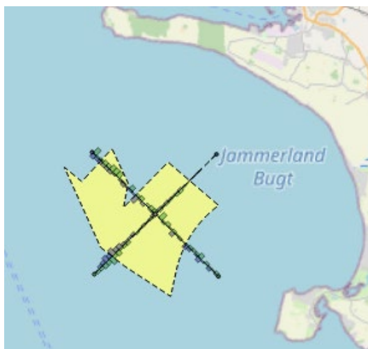
Figure 5-2 Analysis of ships passing two passage lines crossing the wind farm area
