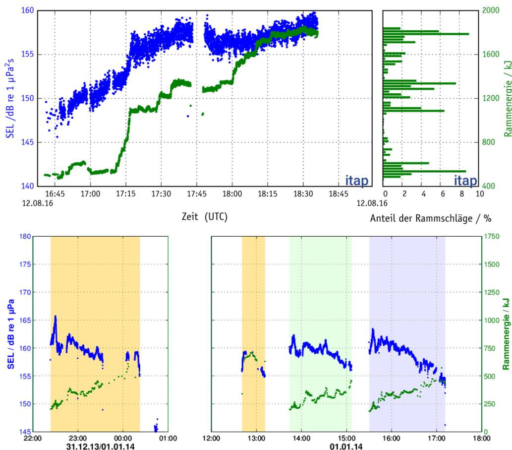
Figure 10: Top: Simple single event level (*SEL*) as a function of time (blue line) and the blow energy used (green line) for a typical monopile installation in the North Sea.
