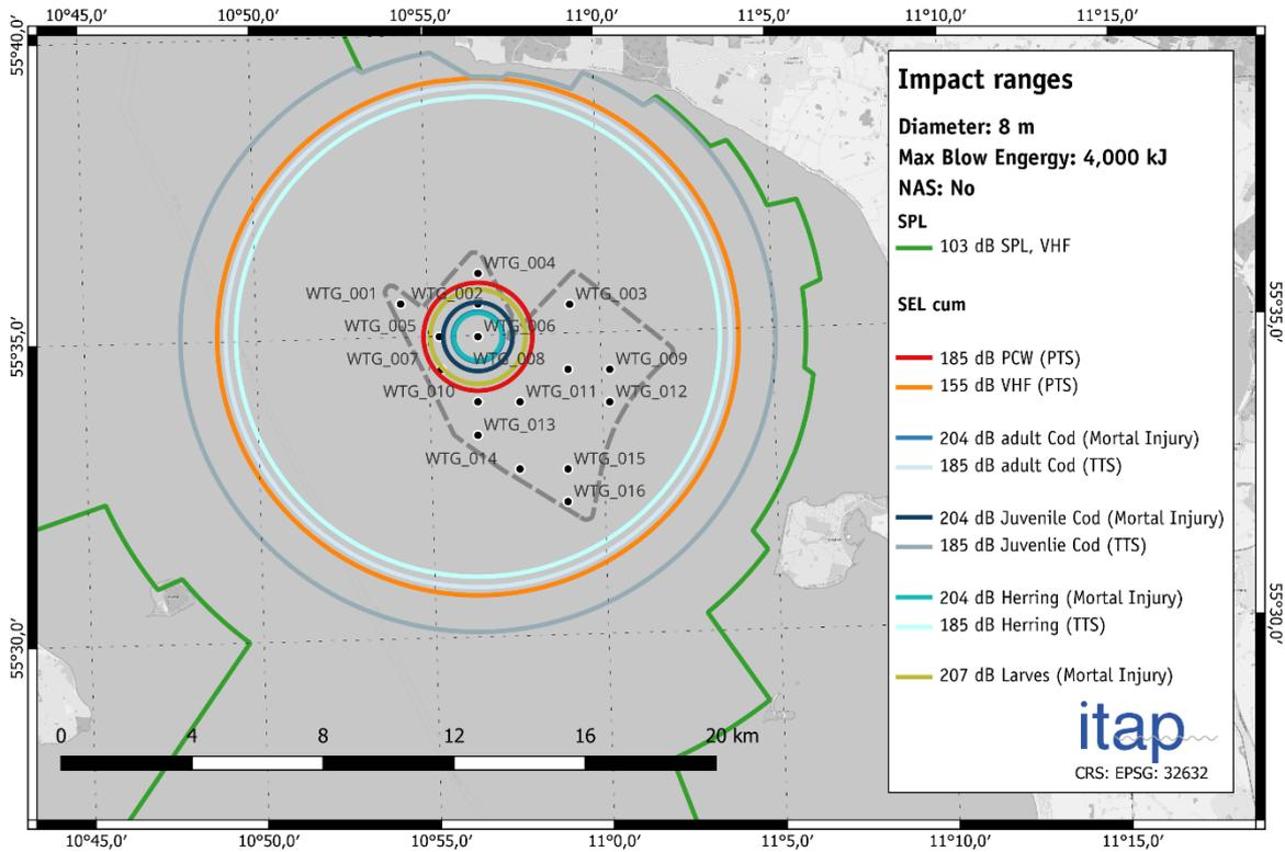
Figure 13: Impact ranges during the installation of the 8.00 m monopile foundation at WTG06 (preferred project design) with a maximum blow energy of 4,000 kJ and a piling sequence of 3,424 blows without noise abatement system (unmitigated – no NAS). The transmission loss estimated for 165° direction (Annex 1) used for all directions and water depths > 5 m.
