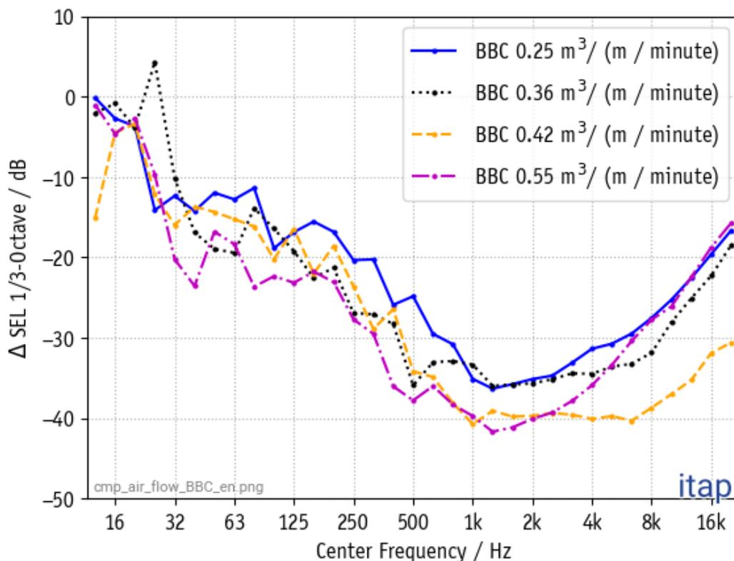
Figure 14: Resulting averaged noise reduction (transition loss) from the test measurements according to the (DIN 45653 2017) with a double Big Bubble Curtain (DBBC) with different supplied air volumes.
