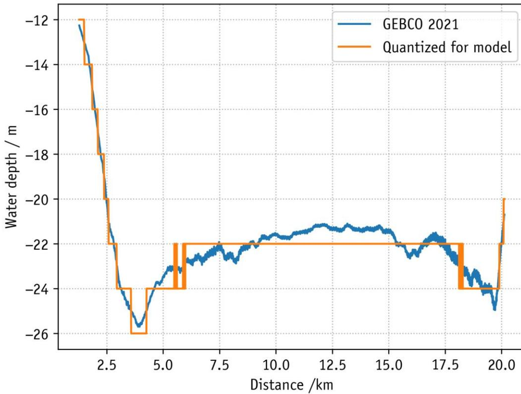
Figure 17: Waterdepth in 165° directions from WTG18/20 (Alternative 1 and 2). Blue: Waterdepth according to GEBCO 2021 and orange: Quantized in 2 m steps used for modeling.
