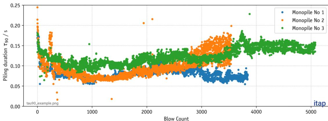
Figure 9: Pile-driving duration  $\tau_{90}$  of single strikes for three different monopile installations in accordance with de Jong et al. (2011).
