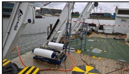
Complete GSO-360 sparker system with HV tow cable, HV junction box and CSP-N Power Supply.
