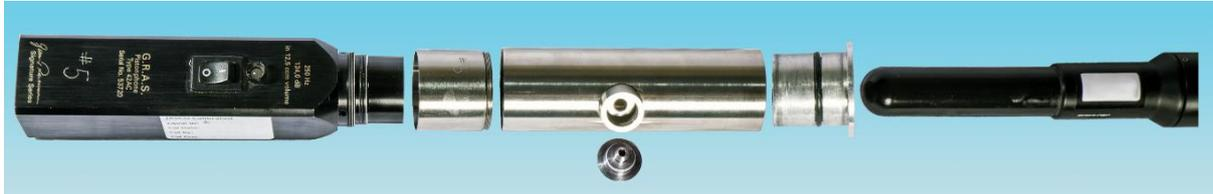
Figure B-1. Split view of a G.R.A.S. 42AC pistonphone calibrator with an M36 hydrophone.
