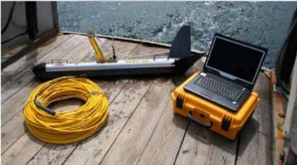
**The 4200 Series** is a versatile side scan sonar system that can be configured for almost any survey application from shallow to deep water operations. The 4200 utilizes EdgeTech's Full Spectrum<sup>®</sup> CHIRP technology to provide crisp, high resolution imagery at ranges up to 50% greater than non-CHIRP systems; thus allowing customers to cover larger areas and save money spent on costly surveys.
