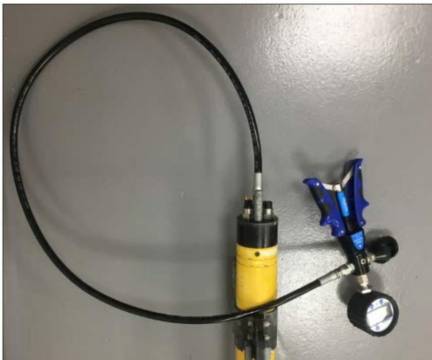
Figure 8.2: Pressure Gauge Connected to a G882 Magnetometer
