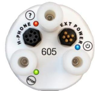
After the AMAR has been powered on for 10 minutes, the LEDs go off to conserve power. For related information, see [Re-activating the LEDs to check the AMAR's status](#) on page 7.
