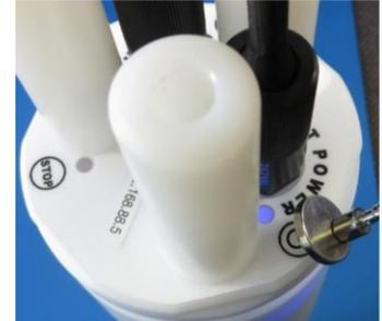
Figure 6: AMAR turn on sequence, taken from the current version of the manual.
