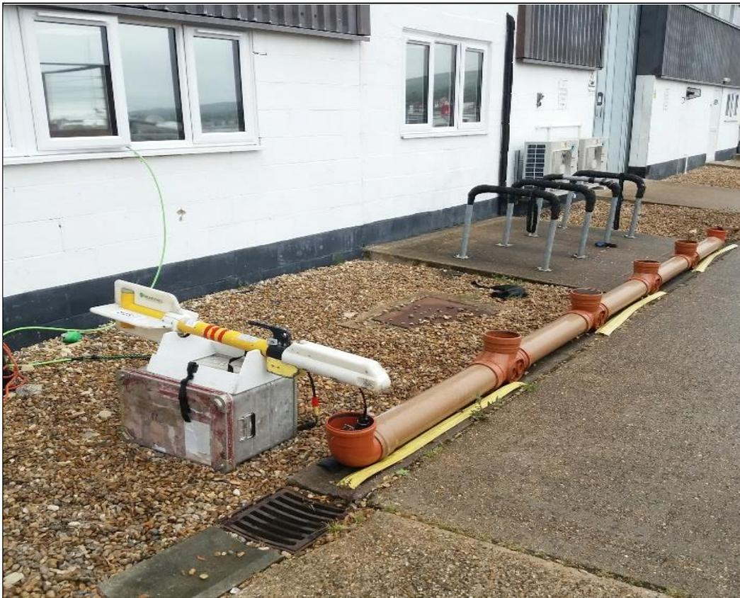
Figure 8.1: Example of Altimeter Verification Setup
