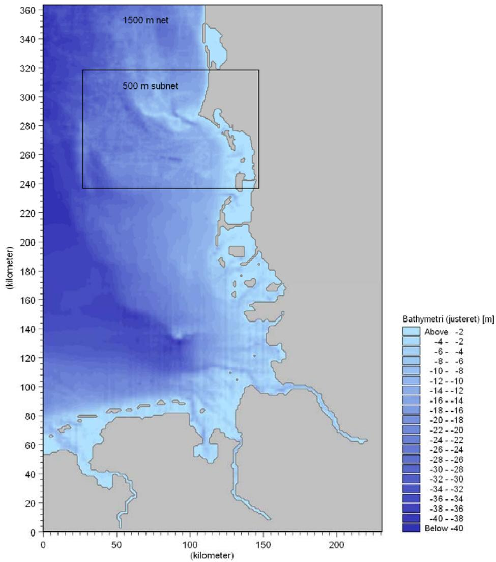
Figure 3.11. Hydrodynamic bathymetry model showing the core fine-scale area around Horns Rev nested into a larger-scale area.
