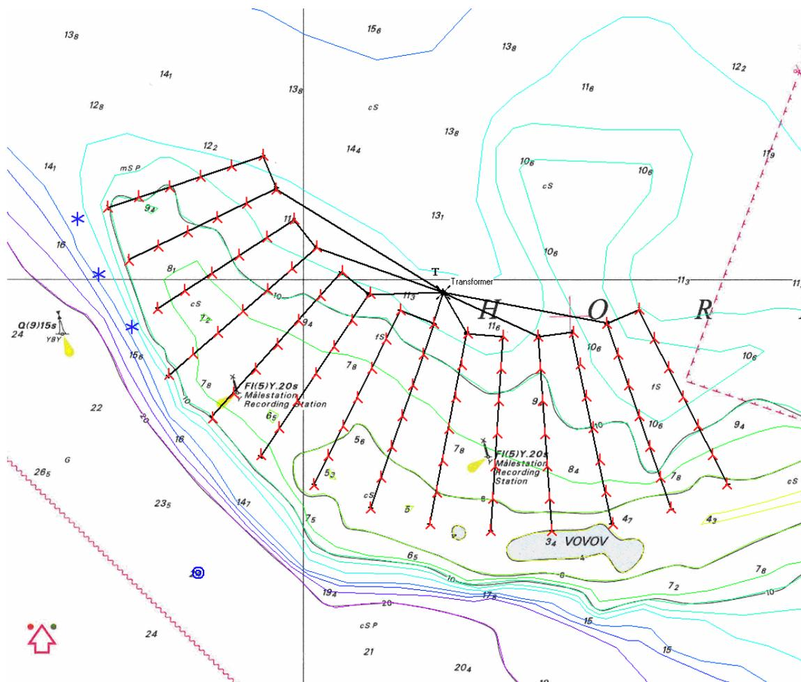
Figure 2.3 Positioning sketch plan for Horns Rev 2 South Offshore Wind Farm showing 95 2.3 MW turbines, 3 test turbines and the transformer.
