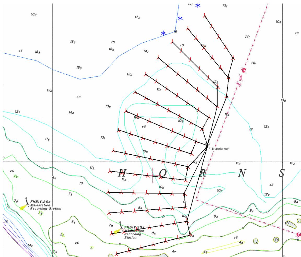
Figure 2.2 Positioning sketch plan for Horns Rev 2 North Offshore Wind Farm showing 95 2.3 MW turbines, 3 test turbines and the transformer.
