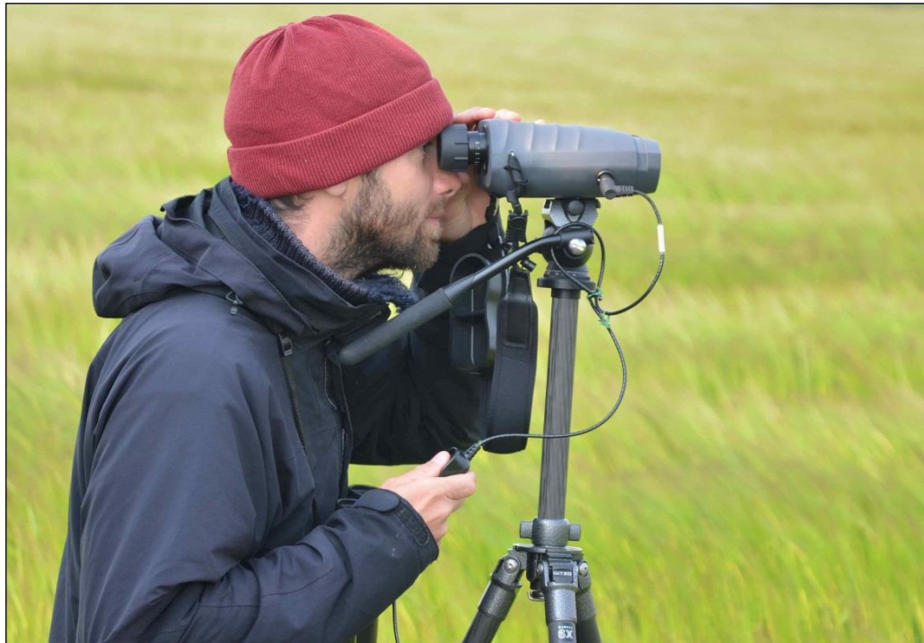
Figure 5-4. Tracking migrating raptor with laser rangefinder. When pushing the button the bird's position and altitude is stored.
