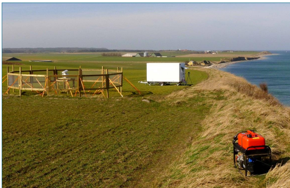
Figure 5-2. The observation site at Gjerrild (21 m above sea level) with the radar surrounded by a “clutter fence” to the left.
