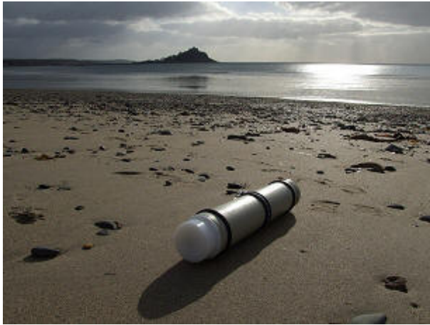
Figure 3-3. The C-POD used in the project.
