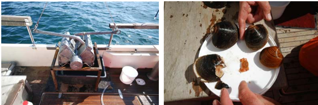
Figure 3-3 Left: Van Veen grab sampler (0.1m 2 ) used to collect samples for analyses of benthic fauna and sediment. Right: Large specimens of Icelandic cyprine ( Arctica islandica ), which was a problem for sampling at many stations.
