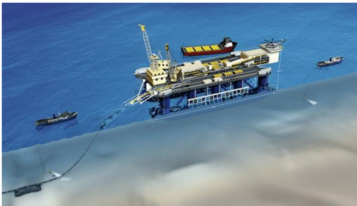
Figure 6-15 The S-lay pipe-lay vessel and survey support vessels.
