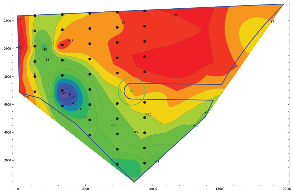
Figure 13. Suggested layout for the 10.0MW wind turbine at Horns Rev 3, located most westerly in the area.
