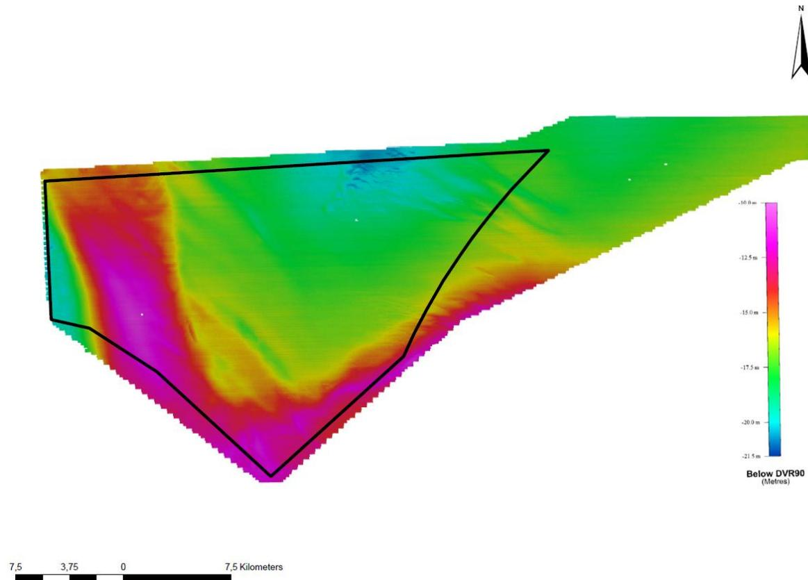
Figure 2. Bathymetric map of the Horns Rev 3 area showing depths below DVR90 as graded colour. The map is based upon the Geophysical survey in 2012. The black line encircles the pre-investigation area of 160km<sup>2</sup>.
