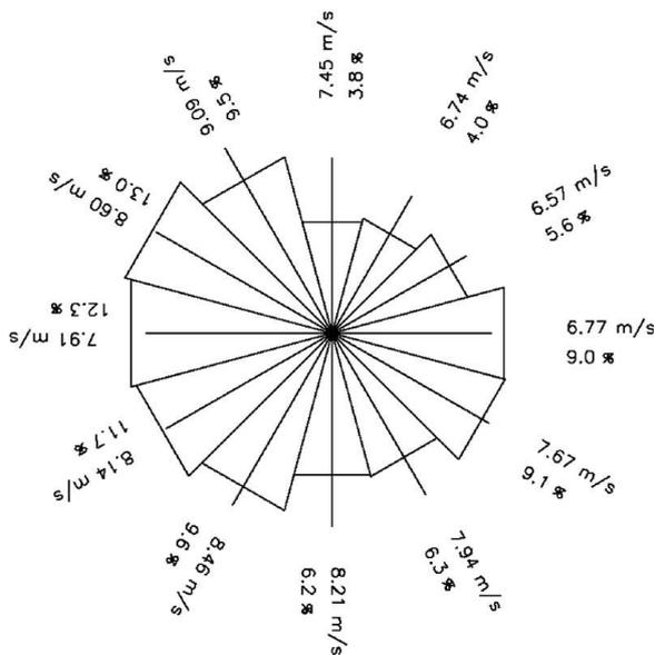
Figure 4. Wind rose from the Horns Rev (from NASA/Risø).
