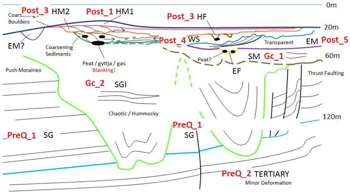
Figure 5. Horns Rev 3 Geological Model (COWI February 2014)
