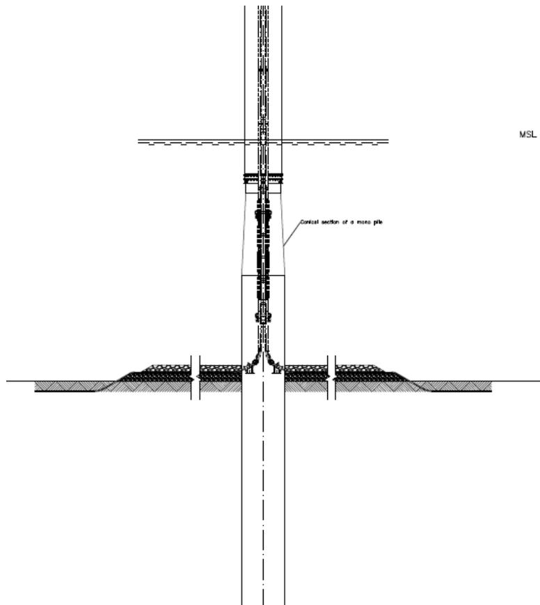
The principal illustration above shows the conical part of the mono-pile. The mono-pile section above the conical part has a smaller outer diameter than the part of the mono-pile below the conical part. The outer diameter of the pile above the conical part then allows for a transition piece with an inner diameter smaller than the outer diameter of the imbedded pile – taken the length of the pile section above the conical part into account compared to the length of the transition piece.
