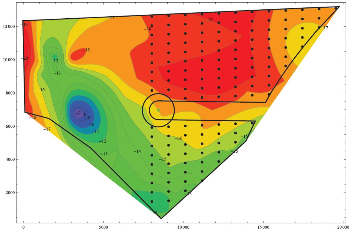
Figure 5. Suggested layout for the 3.0MW turbine at Horns Rev 3, closest to shore.
