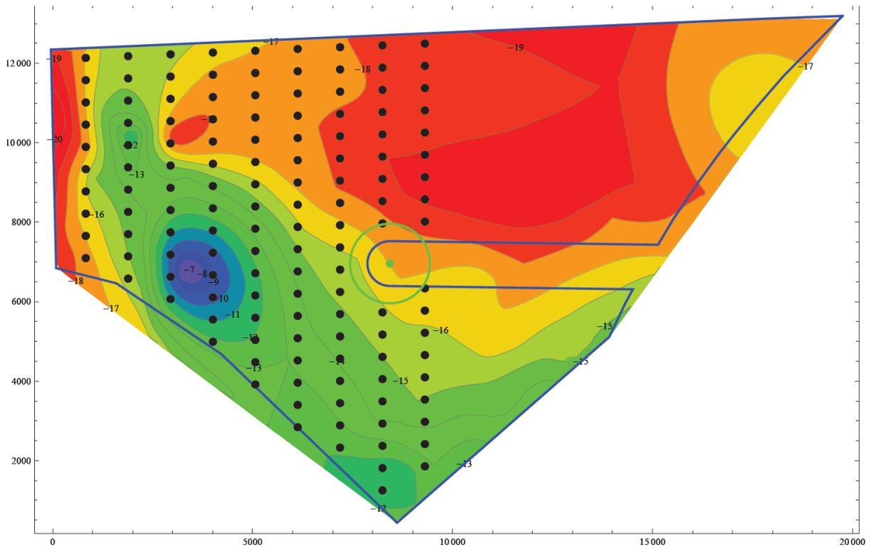
Figure 11. Suggested layout for the 3.0MW turbine at Horns Rev 3, located most westerly in the area.
