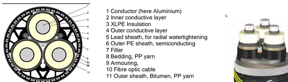
Figure 18. Illustration of a typical export cable. To the left the cross section, and the cable to the right.
