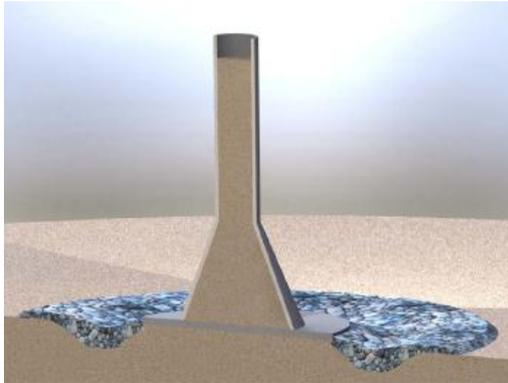
Figure 17. Example of scour protection
