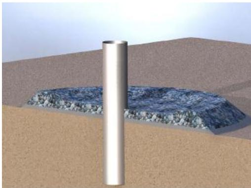
Figure 16. Example of scour protection
