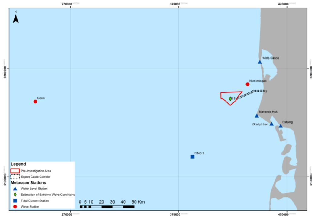
Figure 3.1. Metoccean data stations for Horns Rev 3.
