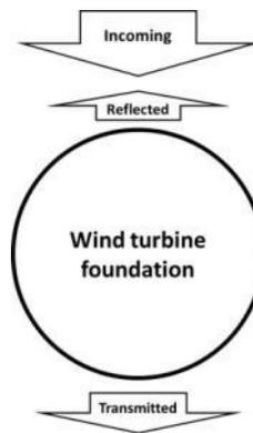
Redistribution of wave energy due to a wind turbine foundation
