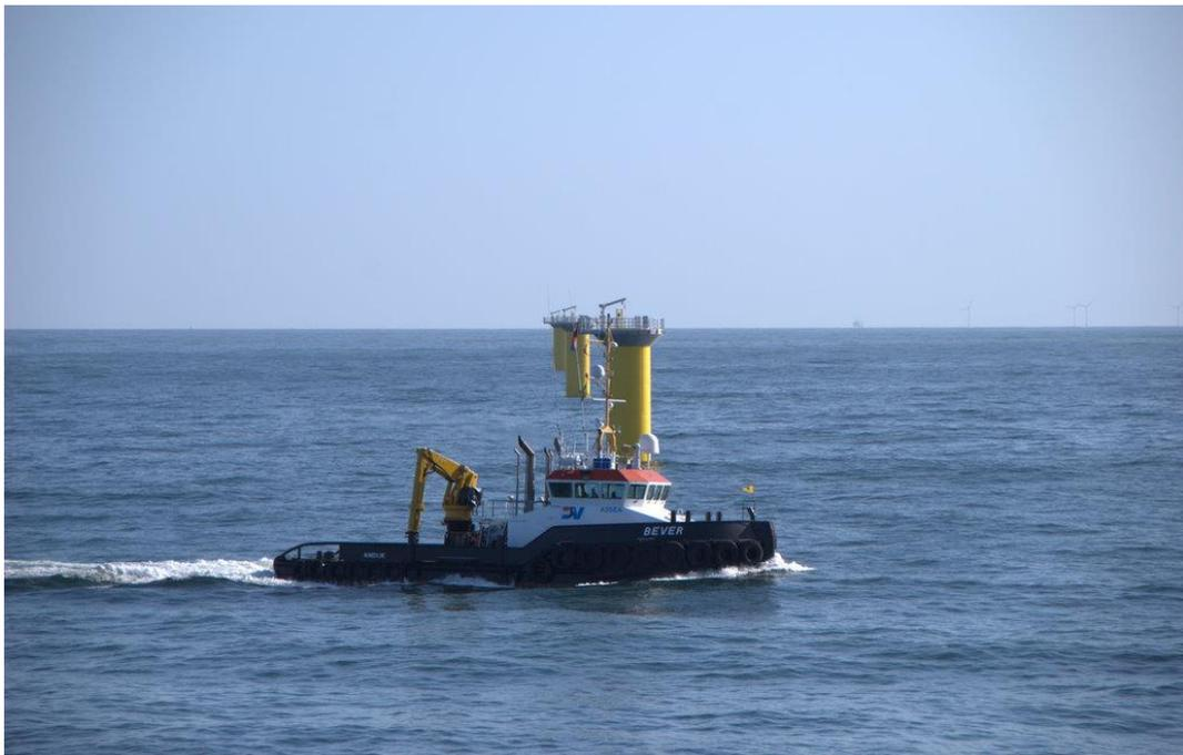
*Foundations ta Horns Rev 2 Offshore Wind Farm*
