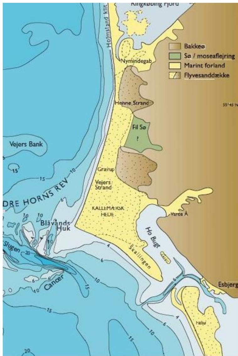
Figure 5.1. Geomorphology of the coastal region landward of Horns Rev 3. Legend: Bakkeø = erosional remnants of Saalian landscape; Sø / moseaflejring = lake and bog deposits; Marint forland = marine foreland; Flyvesanddække = wind deposit sand (Larsen, 2003).
