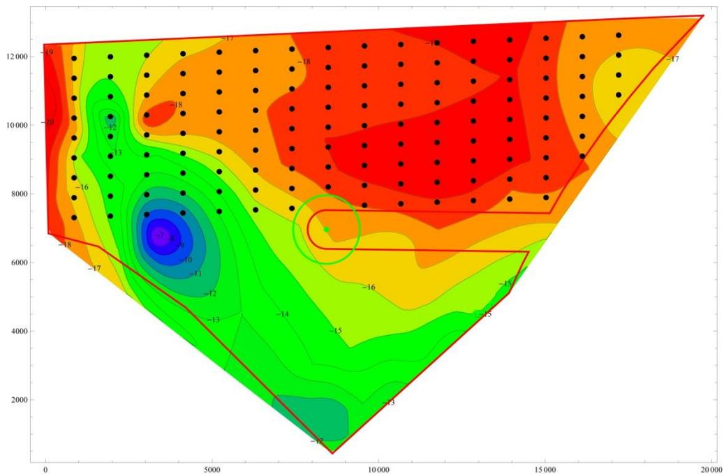
Figure 2.6 Suggested layout for the 3.0 MW wind turbine at Horns Rev 3, located in the centre of the area. Contourlines are colour coded to the nearest 1 m (Note that the coding order is reversed as compared to figure 2.2.).
