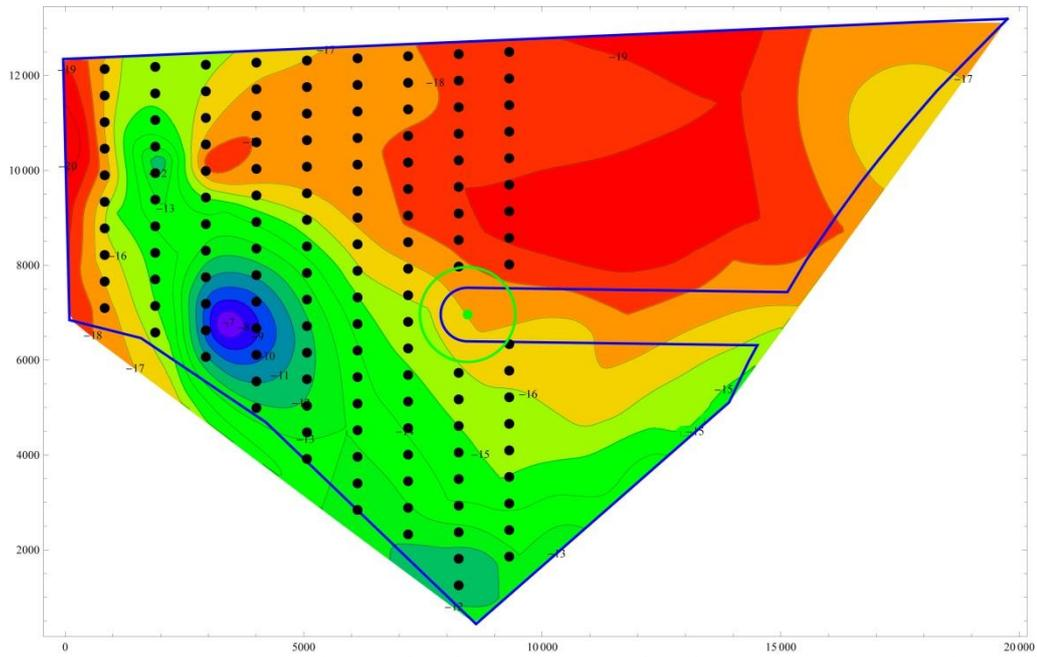
Figure 2.9 Suggested layout for the 3.0 MW wind turbine at Horns Rev 3, located most westerly in the area. Contourlines are colour coded to the nearest 1 m (Note that the coding order is reversed as compared to figure 2.2.).
