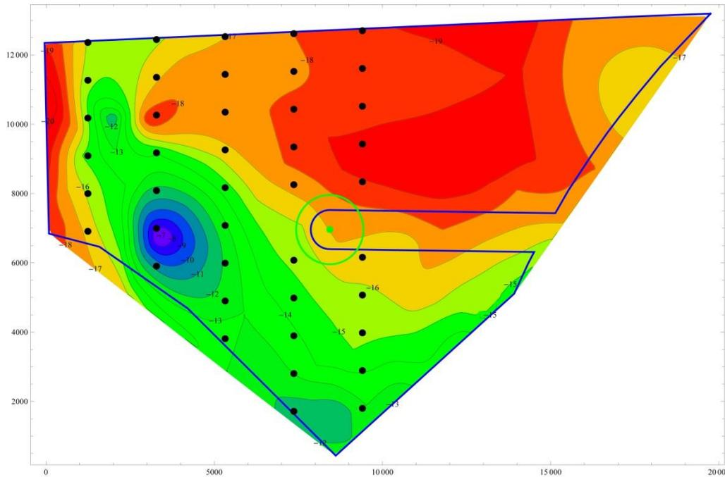
Figure 2.11 Suggested layout for the 10.0 MW wind turbine at Horns Rev 3, located most westerly in the area. Contourlines are colour coded to the nearest 1 m (Note that the coding order is reversed as compared to figure 2.2.).
