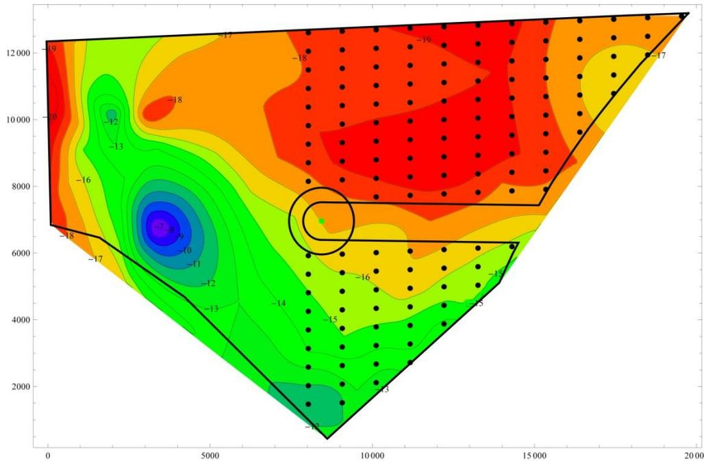
Figure 2.3 Suggested layout for the 3.0 MW wind turbine at Horns Rev 3, closest to shore. Contourlines are colour coded to the nearest 1 m (Note that the coding order is reversed as compared to figure 2.2.).
