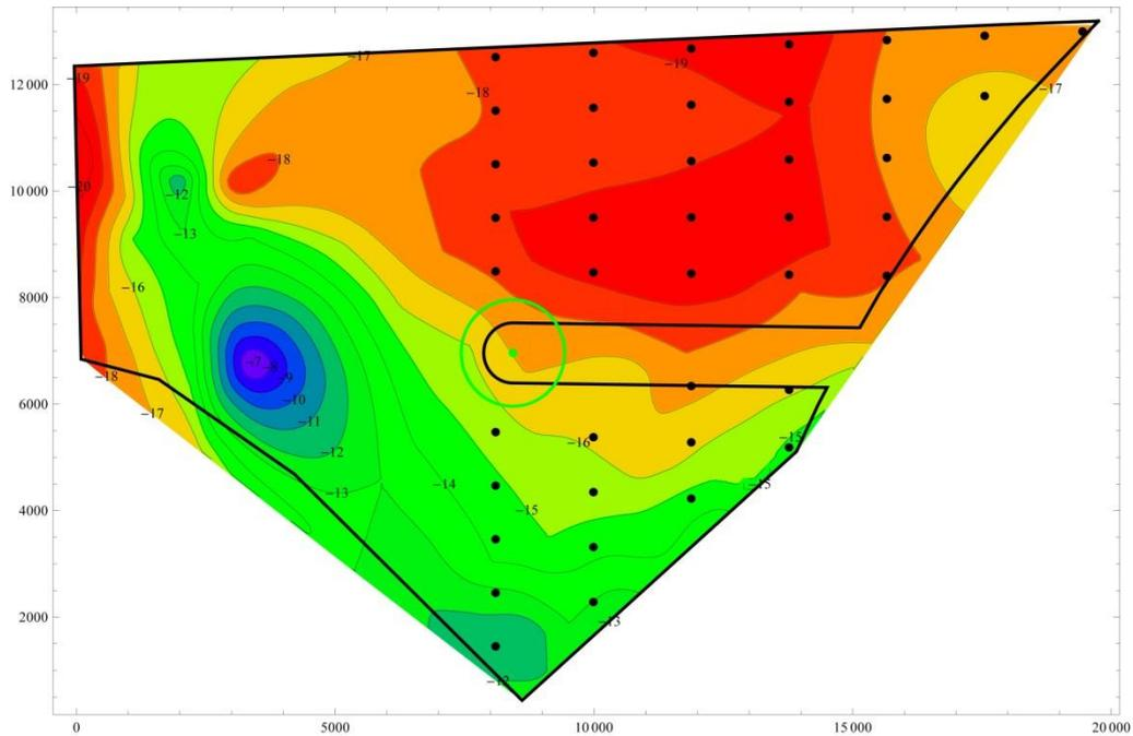
Figure 2.5 Suggested layout for the 10.0 MW wind turbine at Horns Rev 3, closest to shore. Contourlines are colour coded to the nearest 1 m (Note that the coding order is reversed as compared to figure 2.2.).
