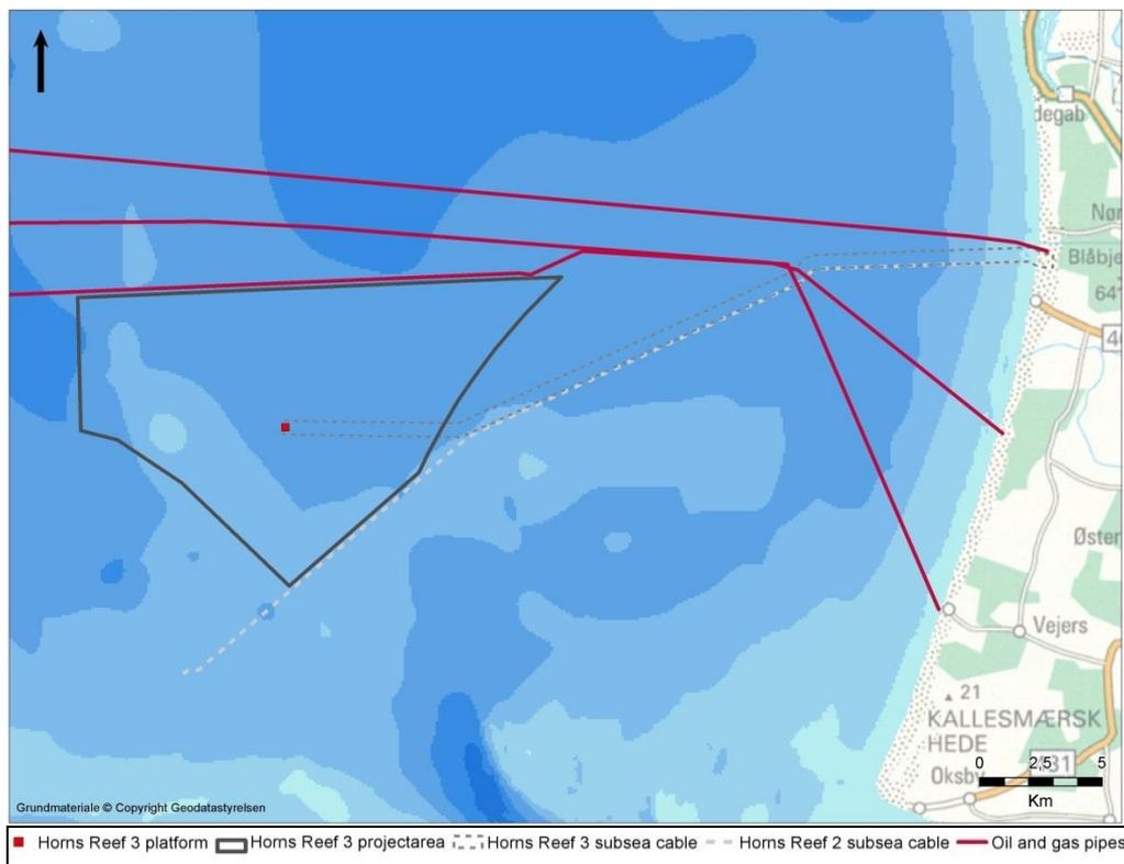
Figure 2.1 Location of the Horns Rev 3 OWF (400 MW) and the projected corridor for export cables towards shore. The area enclosed by the polygon is ca. 150 km<sup>2</sup>. The marked area includes the whole pre-investigation area, i.e. with an overlap of existing cables etc.
