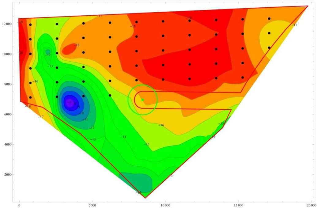
Figure 2.7 Suggested layout for the 8.0 MW wind turbine at Horns Rev 3, located in the centre of the area. Contourlines are colour coded to the nearest 1 m (Note that the coding order is reversed as compared to figure 2.2.).
