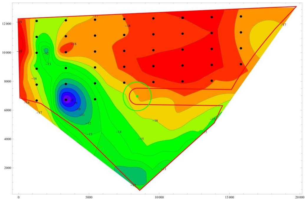
Figure 2.8 Suggested layout for the 10.0 MW wind turbine at Horns Rev 3, located in the centre of the area. Contourlines are colour coded to the nearest 1 m (Note that the coding order is reversed as compared to figure 2.2.).
