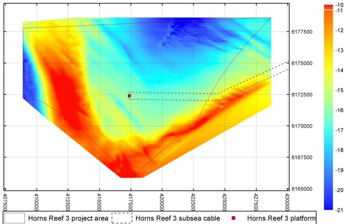
Figure 2.2 Bathymetric map of the Horns Rev 3 area showing depths below DVR90 as graded colour (see column on the right). The map is based upon the Geophysical survey in 2012.
