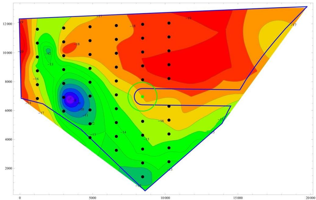
Figure 2.10 Suggested layout for the 8.0 MW wind turbine at Horns Rev 3, located most westerly in the area. Contourlines are colour coded to the nearest 1 m (Note that the coding order is reversed as compared to figure 2.2.).
