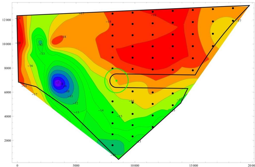
Figure 2.4 Suggested layout for the 8.0 MW wind turbine at Horns Rev 3, closest to shore. Contourlines are colour coded to the nearest 1 m (Note that the coding order is reversed as compared to figure 2.2.).
