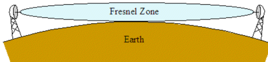
Figure 6.1. The first Fresnel zone is defined as an ellipsoid between the two antennas within which all possible propagation paths are within less than half a wavelength in total length from the direct path (RABC, 2010).
