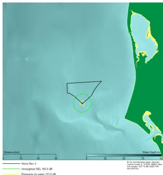
Figure 4.5 Contour plot showing the estimated impact ranges for the identified TTS criteria for marine mammals from installing a 10 m diameter pile using a maximum blow energy of 3000 kJ at the South modelling location.
