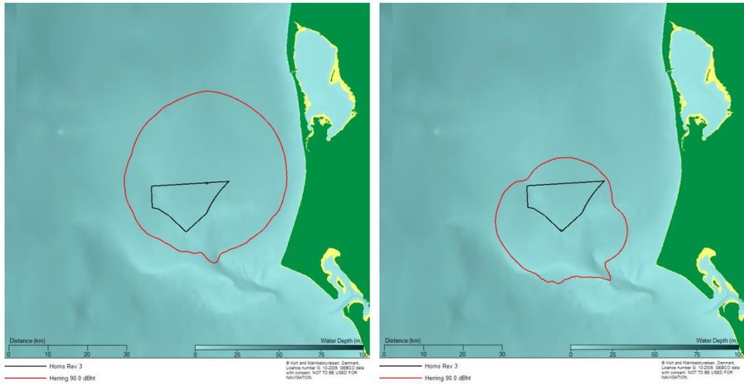
Figure 4.12 Contour plot showing the estimated levels of noise in terms of  $dB_{ht}$  for herring from installing a 10 m diameter pile using a maximum blow energy of 3000 kJ at the North East (left) and South (right) modelling location.
