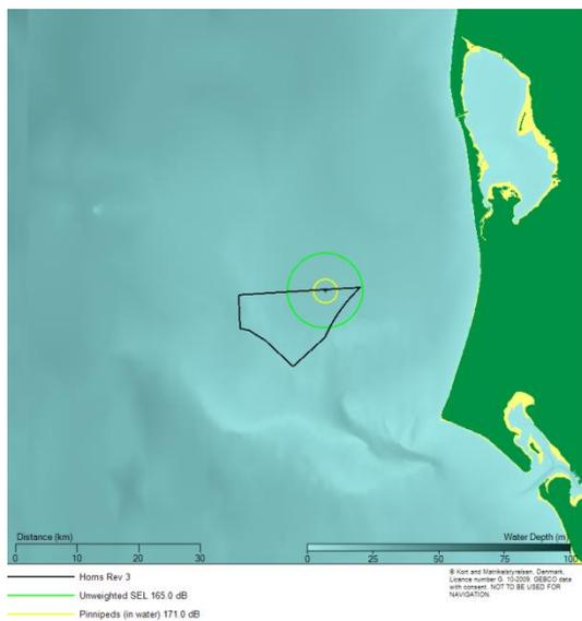
Figure 4.4 Contour plot showing the estimated impact ranges for the identified TTS criteria for marine mammals from installing a 10 m diameter pile using a maximum blow energy of 3000 kJ at the North East modelling location.
