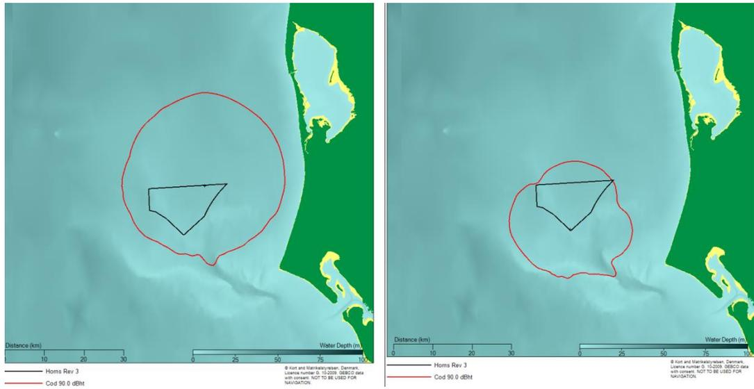
Figure 4.10 Contour plot showing the estimated levels of noise in terms of  $dB_{ht}$  for cod from installing a 10 m diameter pile using a maximum blow energy of 3000 kJ at the North East (left) and South (right) modelling location.
