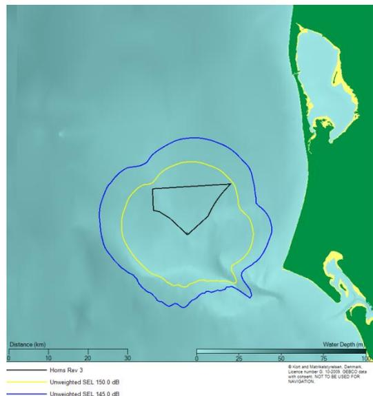
Figure 4.9 Contour plot showing the estimated impact ranges for the identified unweighted SEL behavioural effect criteria for marine mammals from installing a 10 m diameter pile using a maximum blow energy of 3000 kJ at the South modelling location.
