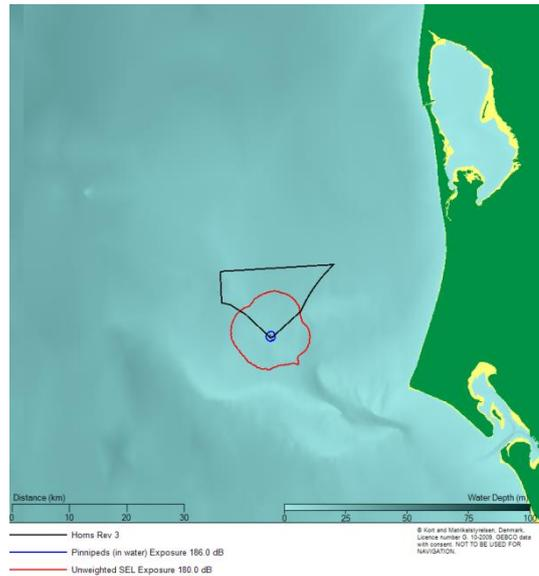
Figure 4.3 Contour plot showing the estimated impact ranges for the identified PTS criteria for marine mammals from installing a 10 m diameter pile using a maximum blow energy of 3000 kJ at the South modelling location.
