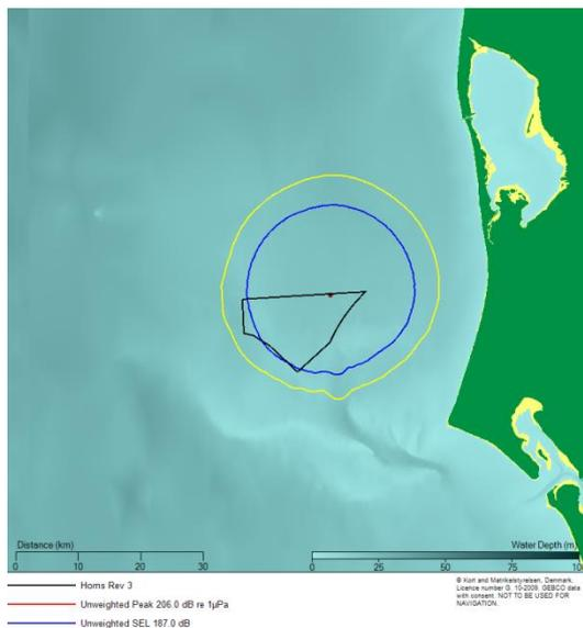
Figure 4.6 Contour plot showing the estimated impact ranges for the identified injury criteria for fish from installing a 10 m diameter pile using a maximum blow energy of 3000 kJ at the North East modelling location.
