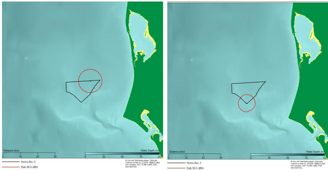
Figure 4.11 Contour plot showing the estimated levels of noise in terms of  $dB_{ht}$  for dab from installing a 10 m diameter pile using a maximum blow energy of 3000 kJ at the North East (left) and South (right) modelling location.
