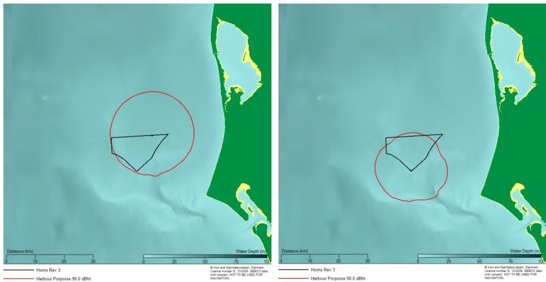
Figure 4.13 Contour plot showing the estimated levels of noise in terms of  $dB_{ht}$  for harbour porpoise from installing a 10 m diameter pile using a maximum blow energy of 3000 kJ at the North East (left) and South (right) modelling location.
