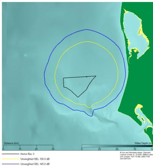
Figure 4.8 Contour plot showing the estimated impact ranges for the identified unweighted SEL behavioural effect criteria for marine mammals from installing a 10 m diameter pile using a maximum blow energy of 3000 kJ at the North East modelling location.
