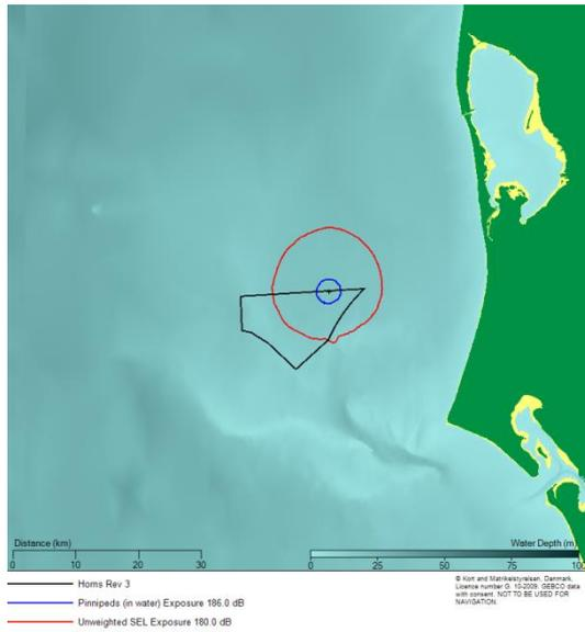
Figure 4.2 Contour plot showing the estimated impact ranges for the identified PTS criteria for marine mammals from installing a 10 m diameter pile using a maximum blow energy of 3000 kJ at the North East modelling location.
