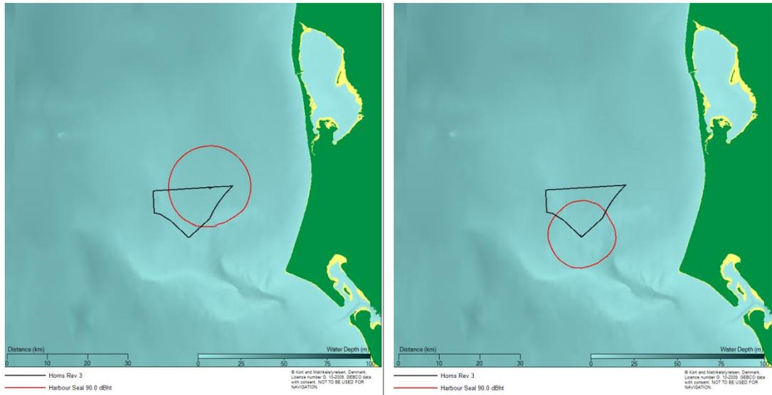
Figure 4.14 Contour plot showing the estimated levels of noise in terms of  $dB_{ht}$  for harbour seal from installing a 10 m diameter pile using a maximum blow energy of 3000 kJ at the North East (left) and South (right) modelling location.
