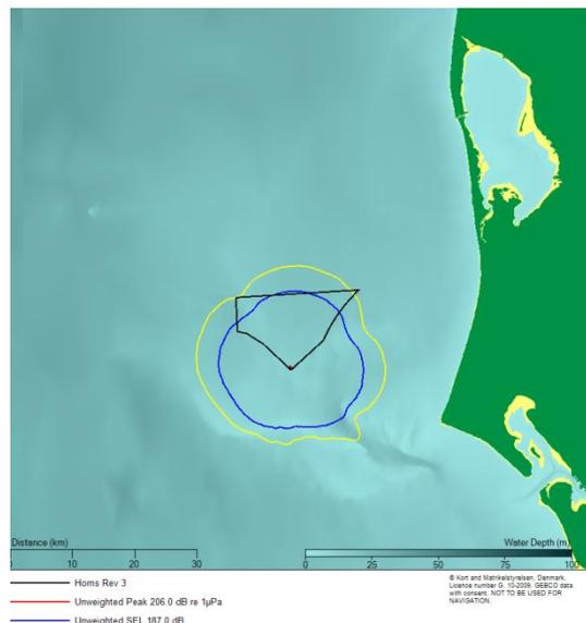
Figure 4.7 Contour plot showing the estimated impact ranges for the identified injury criteria for fish from installing a 10 m diameter pile using a maximum blow energy of 3000 kJ at the South modelling location
