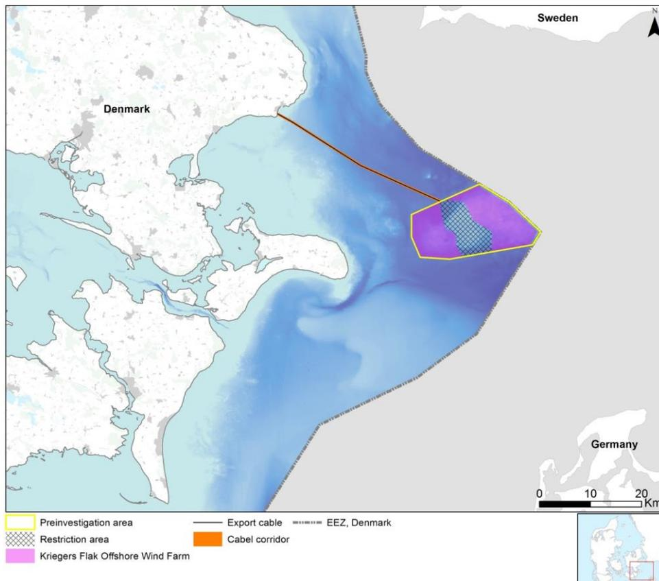
**Figure 3-1** The planned location of Kriegers Flak Offshore Wind Farm (600 MW) in the Danish territory. Approximately in the middle of the pre-investigation area an area (ca. 28 km<sup>2</sup>) is reserved for sand extraction with no permission for technical OWF components to be installed (hatched area). The cable corridor shown on the figure contains two export cables. The final positions of the cables within the cable corridor have not yet been determined.
