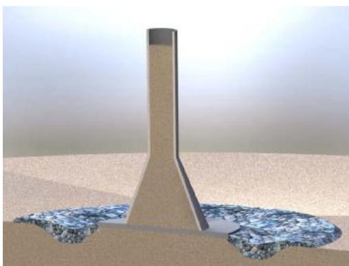
Figure 3-5 Example on scour protection for a concrete gravity base (drawing: Rambøll).
