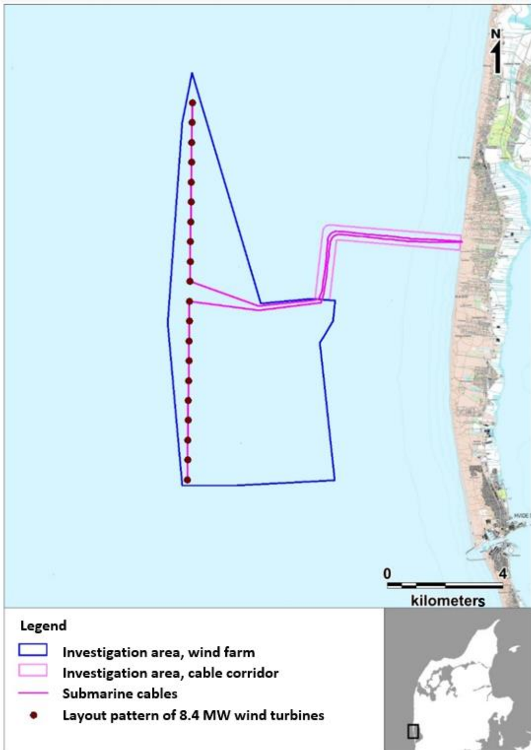
Figure 1-1. This figure shows the layout pattern for the Vesterhav Syd offshore wind project. It also shows the concession site boundary in which Vattenfall is allowed to erect the turbines. This is also the area where a considerable number of environmental surveys have been conducted (the concession area/the survey area).
