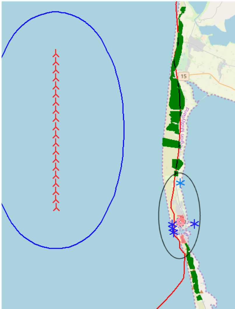
Figure 10. Overview map with the identified areas where the impact at neighbors to operating wind turbines should be considered (Cottage zones marked with green color).
