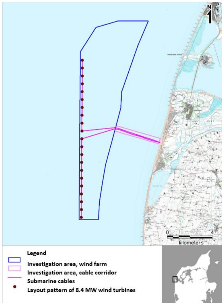
Figure 1-1. This figure shows the layout pattern for the Vesterhav Nord offshore wind project. It also shows the concession site boundary in which Vattenfall is allowed to erect the turbines. This is also the area where a considerable number of environmental surveys have been conducted (the concession area/the survey area).
