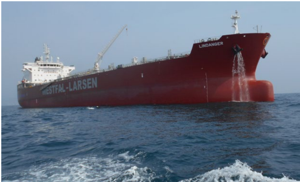
Figure 23 Lindanger, a 50,000 DWT tanker with a dual fuel engine that can run on methanol (Courtesy Westfal-Larsen)
