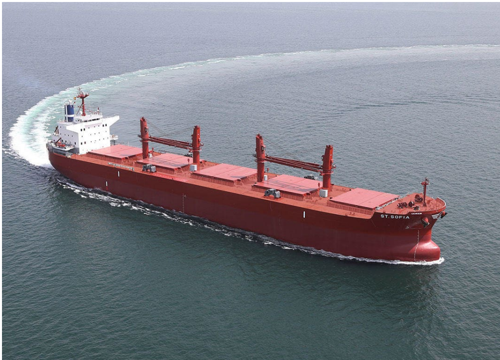
Figure 15 Bulk carrier 60,000 DWT (Copyright Mitsui E&S Shipbuilding)
