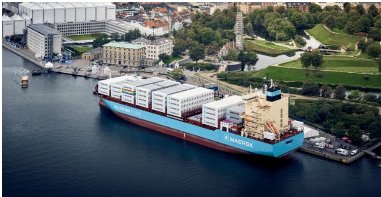
Figure 22 Laura Maersk, the first dual fuel container ship by A.P. Moller-Maersk that can run on methanol (Courtesy State of Green)
