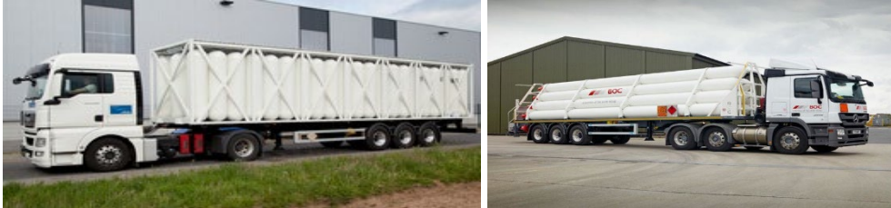
Figure 18: Hydrogen tube trailer types
