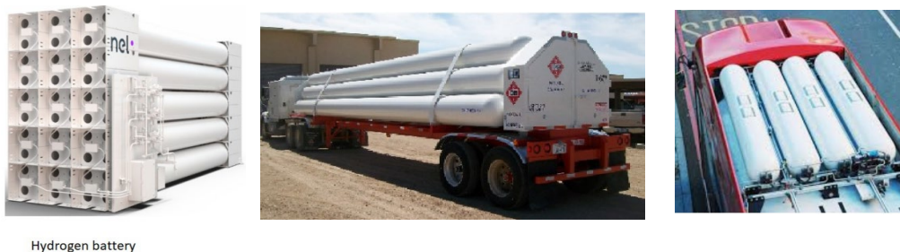
Figure 8: Hydrogen storage, transportation and fuel tank.
