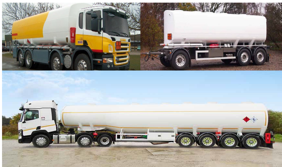
Figure 16: a) Tank, b) trailer, and c) tank trailer (semi-trailer)
