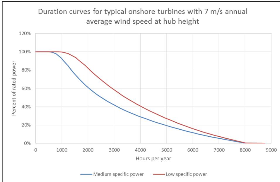
Figure 3 Duration curve for typical modern onshore wind turbines (> 2 MW) located in Denmark (DTU International Energy Report - Wind Energy, 2014). The two curves are based on the V117 3.3 MW (307 W/m<sup>2</sup>) and V126 3.3 MW (265 W/m<sup>2</sup>) wind turbines.
