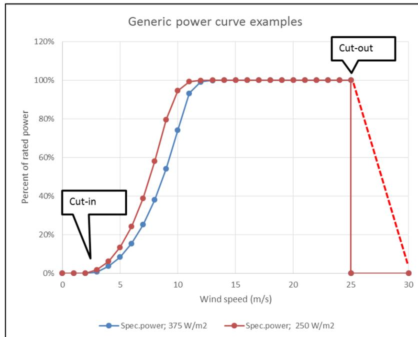
Figure 2 Turbine power curves (Information's from expert workshop held by DEA 27-4-2015). Specific power values refer to e.g. 3 MW with 124m rotor diameter (250 W/m<sup>2</sup>) and 3 MW with 101 m rotor diameter (375 W/m<sup>2</sup>)
