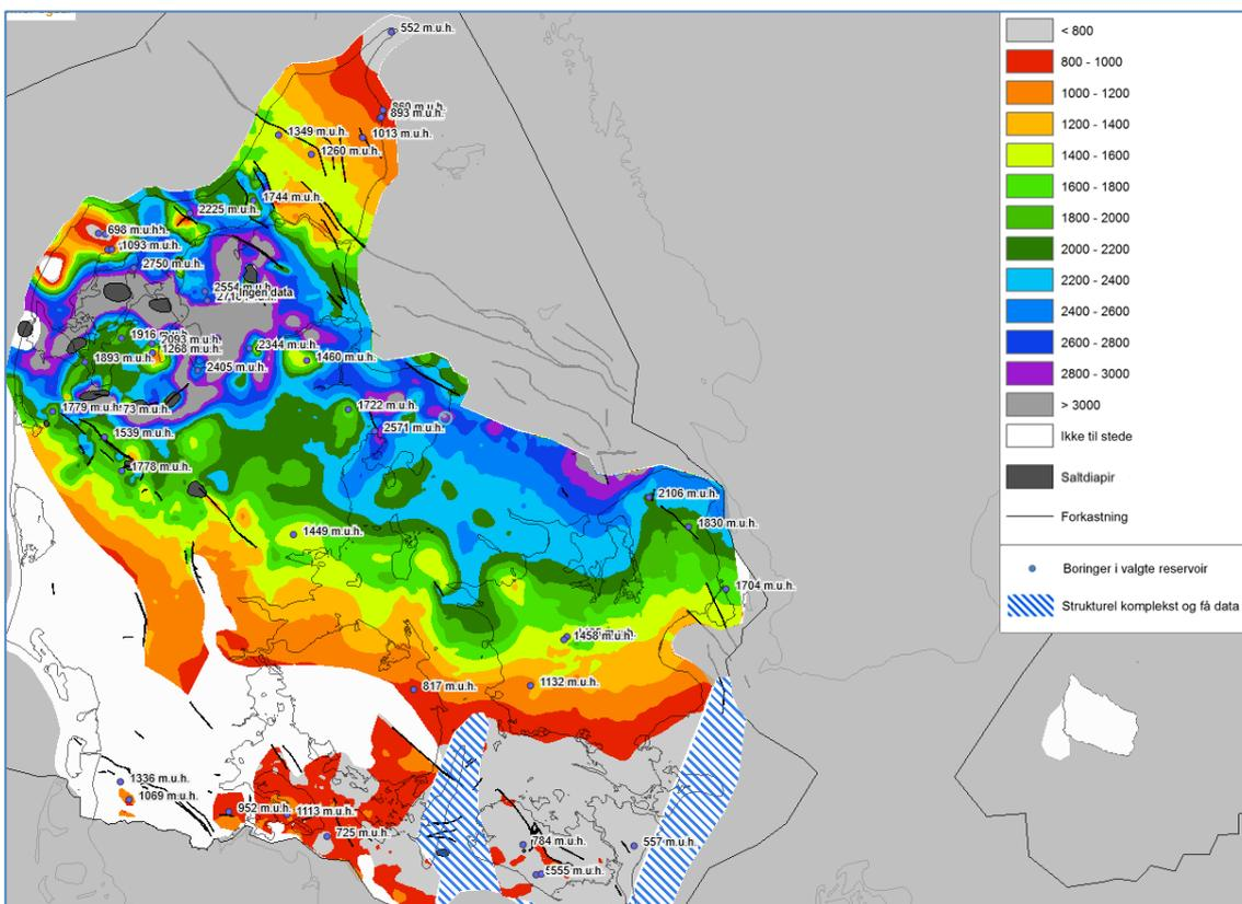
**Figure 0-3: Depth to the top of the Gassum Formation in the Danish area (meters). Locations of wells encountering the Gassum Formation are indicated. Figure from GEUS WebGIS portal <https://dybgeotermi.geus.dk/en/interactive-maps/> selected layers Gassum Fm and "Dybde til top".**
