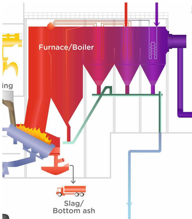
Figure 2 Furnace/boiler system
