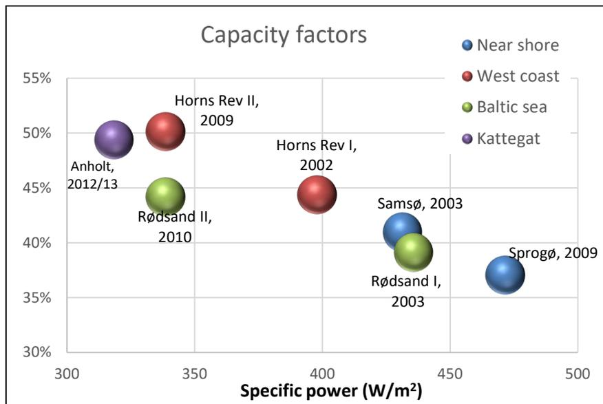
**Figure 7 Capacity Factor shown as function of the Specific Power (W/m<sup>2</sup>) for Danish Offshore wind turbine projects. The three projects most left are the latest ones among the sample. (Figure from previous version of Technology Catalogue, not updated from table above).**
