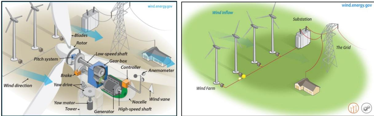
**Figure 1** General turbine technology and electrical system.
