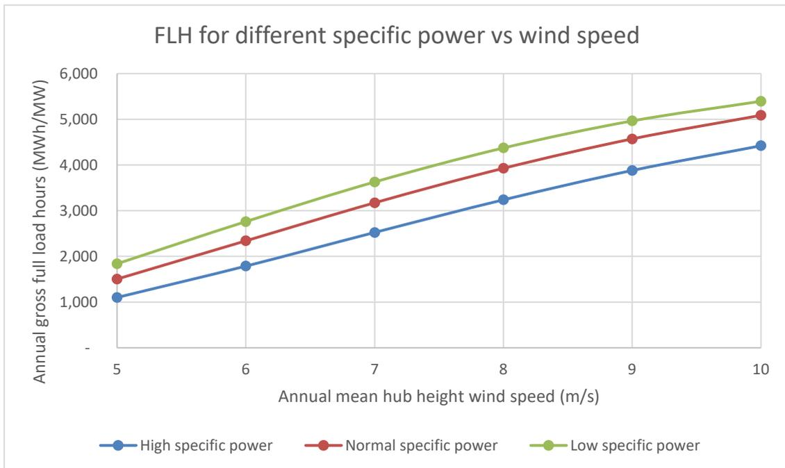
Figure 6 Annual full load hours as a function of mean wind speed at hub height. The examples in the figure are 3 MW with 90m rotor diameter, specific powers are 472 W/m<sup>2</sup> called “high specific power” and 3.3 MW turbines with 112 m and 126 m rotor diameters, specific powers are 335 W/m<sup>2</sup> called “medium specific power” and 265 W/m<sup>2</sup> called “low specific power”.
