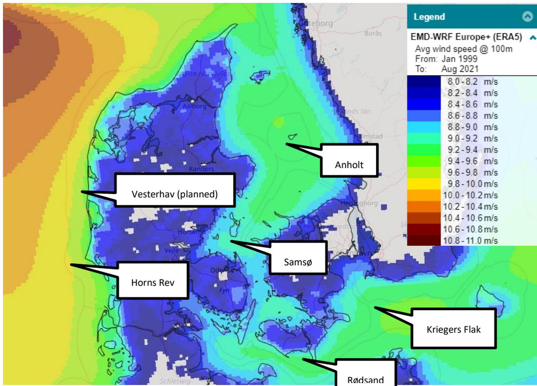
Figure 1 The most recent meso scale model wind data set from EMD International for 100m a.s.l. (above sea level) [1]
