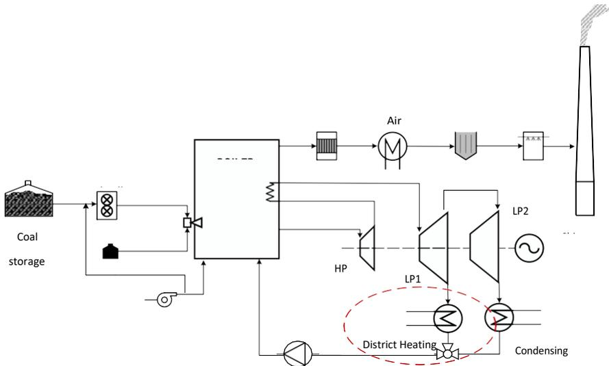
Figure 1: A schematic diagram of an extraction plant.
