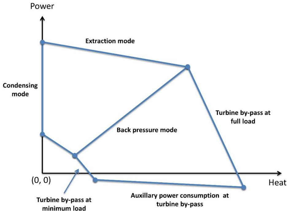
Figure 5 Generic PQ-diagram for extraction CHP
