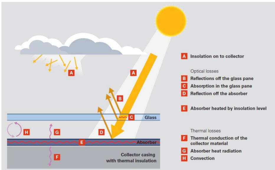
Figure 2 Example of utilisation rate of solar energy and effects influencing the efficiency. [10]
