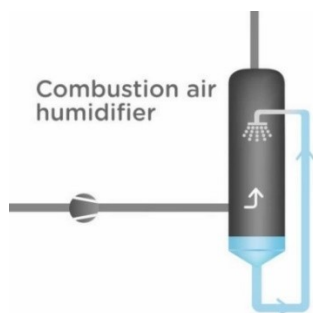
Figure 8 Combustion air humidifier, where water heated by a low-temperature source is evaporated into the combustion air flow.
