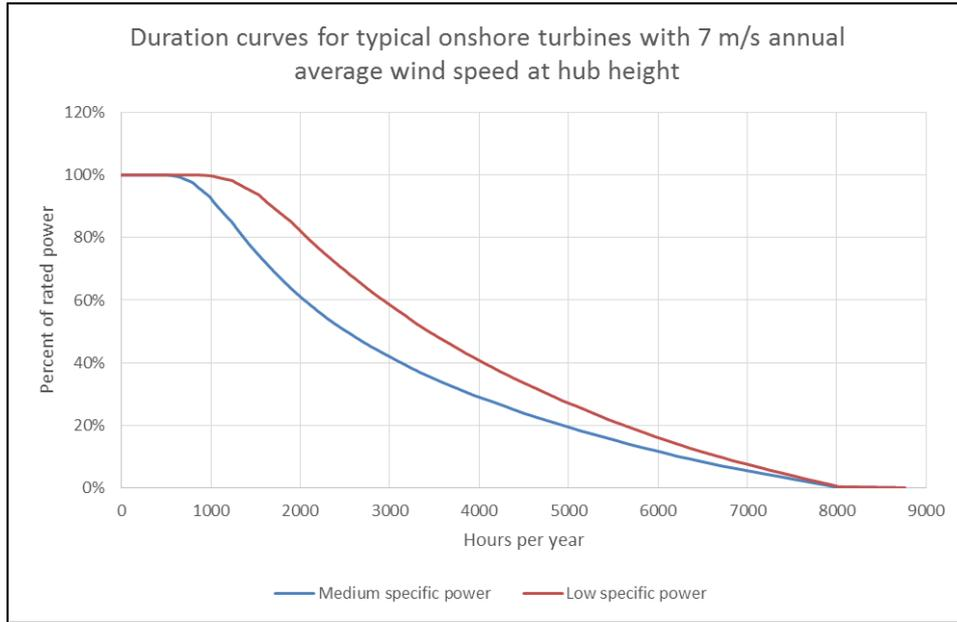
Figure 4 Duration curve for typical modern onshore wind turbines (> 2 MW) located in Denmark (DTU International Energy Report - Wind Energy, 2014). The two curves are based on the V117 3.3 MW (307 W/m<sup>2</sup>) and V126 3.3 MW (265 W/m<sup>2</sup>) wind turbines.
