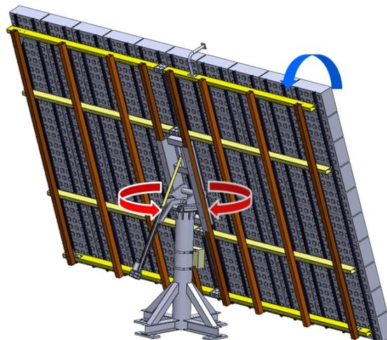
Figure 28 A generic dual axis PV system (Ref. 11)
