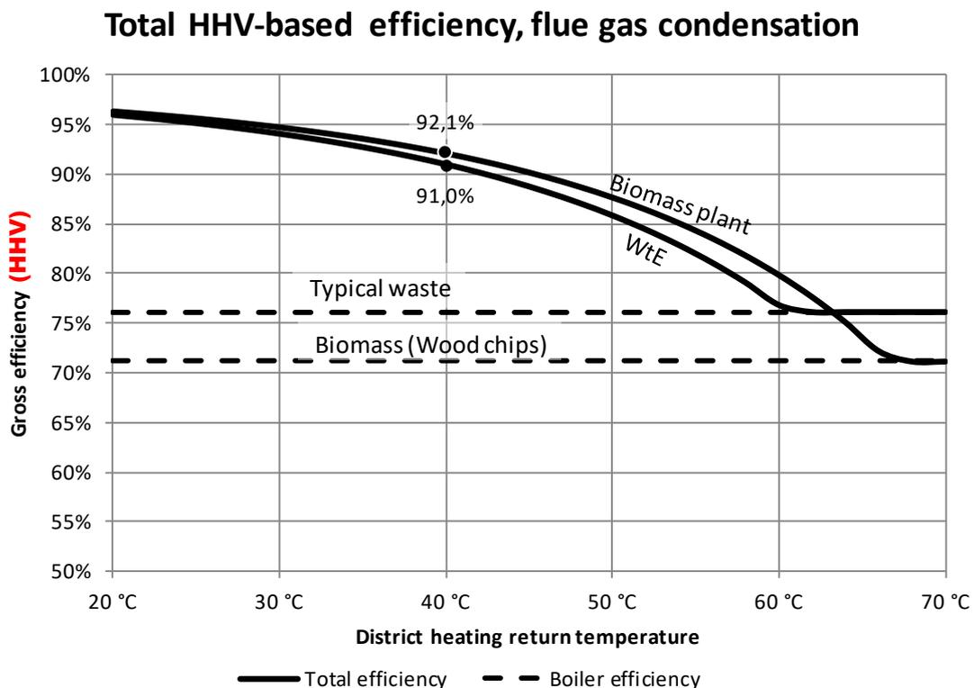
Figure 9. Total HHV-based efficiency estimate for WtE plants<sup>7</sup> and biomass plants<sup>8</sup> given varying DH return temperatures [5] – or temperature of the cold media of a heat pump.
