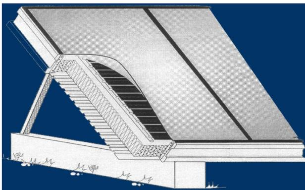
Figure 1 Basic principle of a flat plate solar collector
