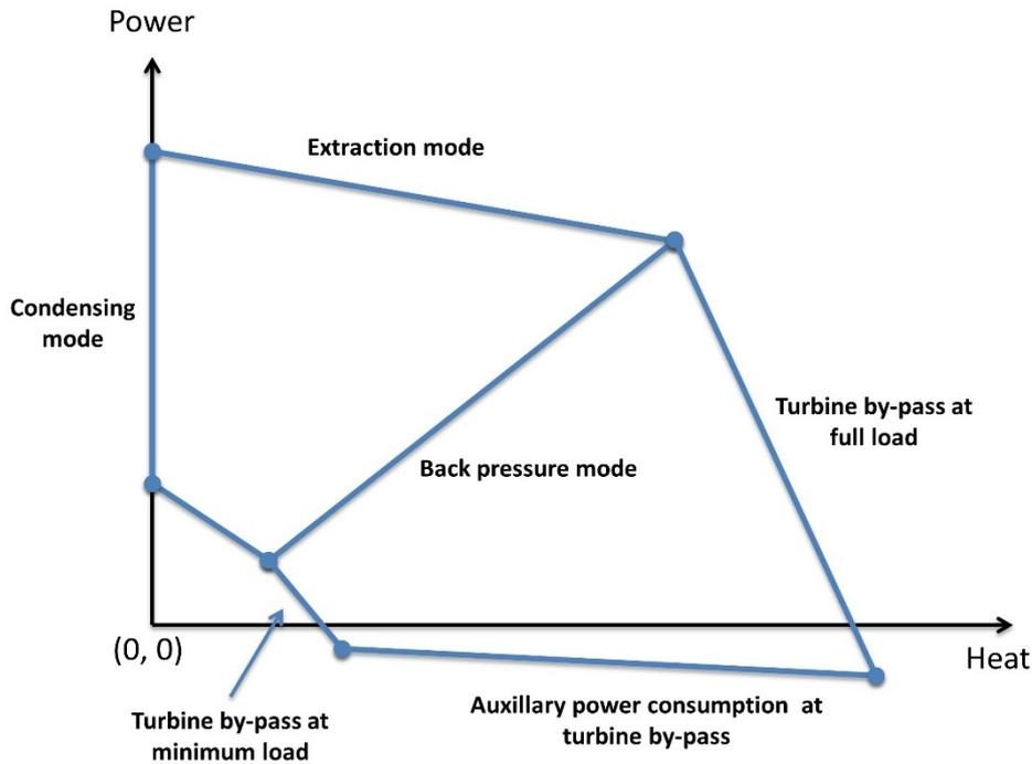
Figure 5 Generic PQ-diagram for extraction CHP
