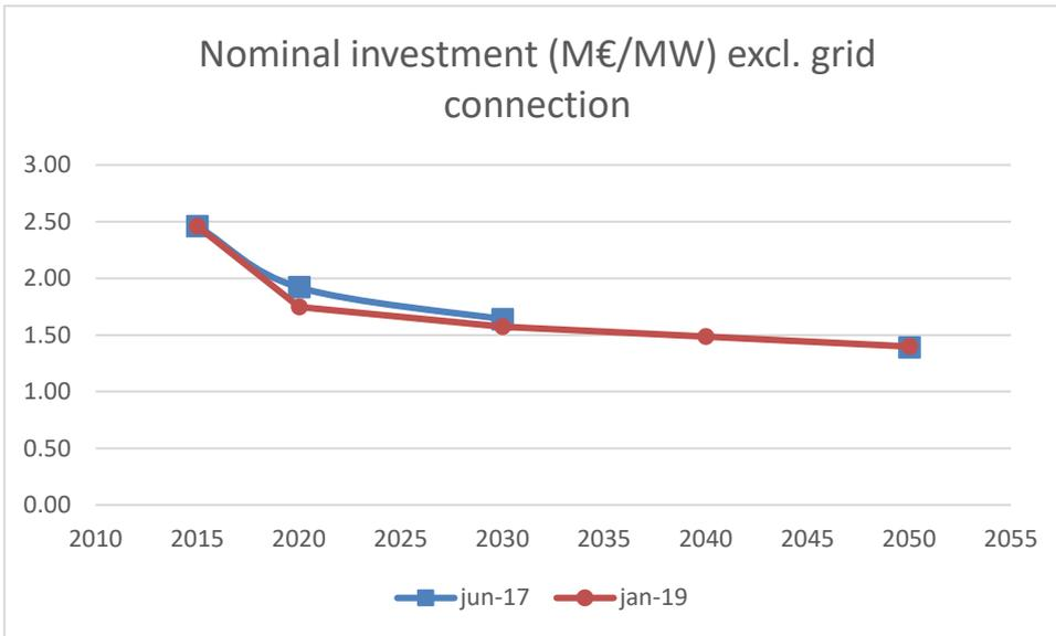
Figure 22 Expected cost development offshore 2019 compared to 2017.
