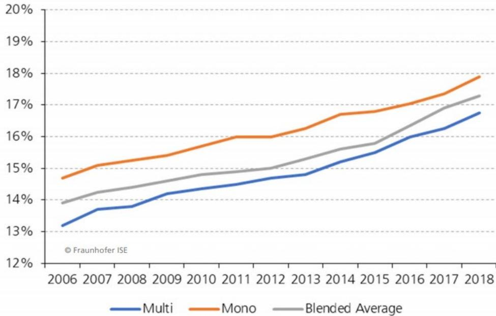
Figure 32 Efficiencies of different cell types (Ref. 9).
