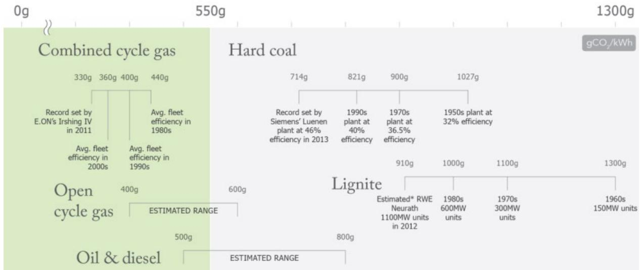
Figure 1 Assessment of carbon-intensity levels by fossil technology [1].
