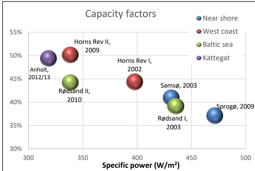
Figure 5: Capacity Factor shown as function of the Specific Power (W/m<sup>2</sup>) for Danish Offshore wind turbine projects. The 3 most left are the latest projects.
