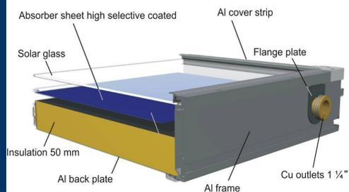
For district heating systems, the collectors are typically installed on the ground in long rows connected in series. In Danish systems, the solar heating system normally takes in the return water and heats it up to the desired forward flow temperature. All plants have the solar collectors mounted on the ground. Ground mount foundations can be concrete blocks, concrete foundations or steel foundations.
