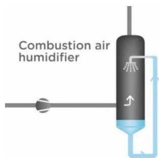
Figure 6 Combustion air humidifier, where water heated by a low-temperature source is evaporated into the combustion air flow.
