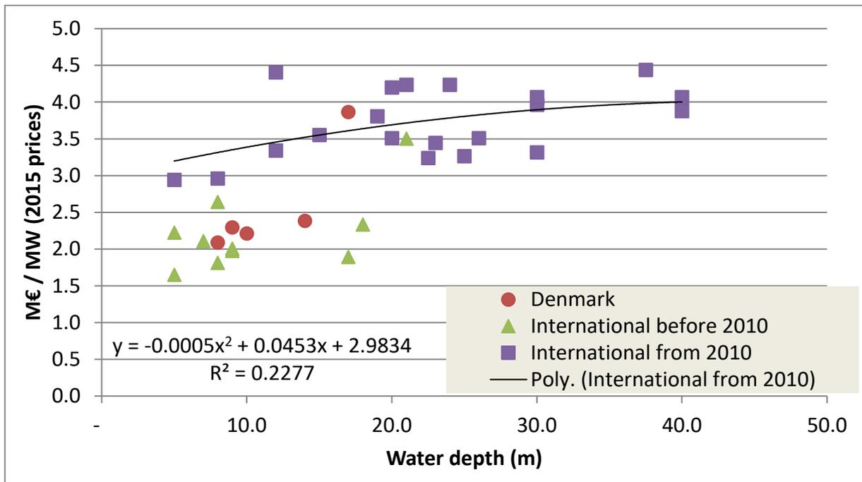
Figure 7: Cost plotted against water depth for 35 realized offshore projects in DK, UK, DE and SE from 2002 to 2014.
