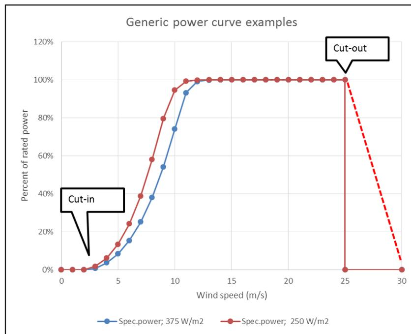
**Figure 3** Turbine power curves (Information's from expert workshop held by DEA 27-4-2015). Specific power values refer to e.g. 3 MW with 124m rotor diameter (250 W/m<sup>2</sup>) and 3 MW with 101 m rotor diameter (375 W/m<sup>2</sup>)
