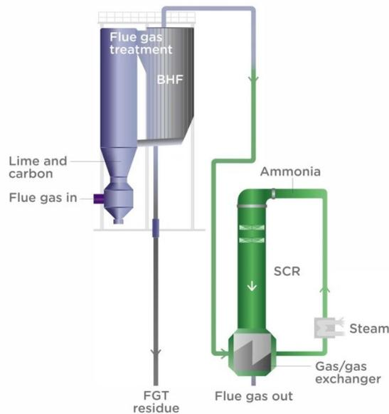
**Figure 4 Flue gas treatment system (dry/semi-dry) including reactor with injection of hydrated lime, a bag house filter and an SCR system with gas/gas heat exchanger, steam reheat, ammonia injection and catalyst.**
