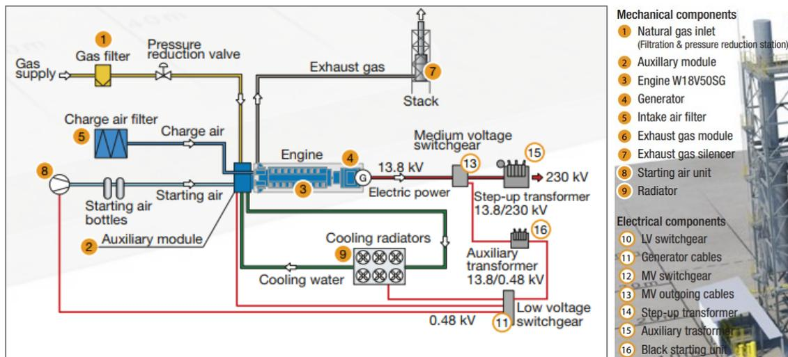
Figure 1 Large engine power plant scheme [16].
