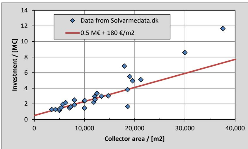
Figure 10 Solar plant investment for Danish SDH projects. The plant in the upper right corner is "Dronninglund" with 37,573 m<sup>2</sup> which includes a seasonal heat storage – and the investment for that is 2.4 M€ (see the section below on the seasonal heat storage), bringing this plant closer to the red line [5].
