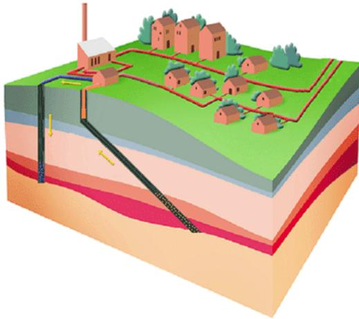
Figure 1: The principle of a doublet system [7]
