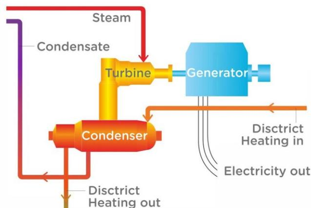
Figure 3 Turbine/generator system
