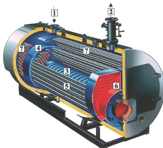
**Figure 1 Typical flue gas tube boiler for the power range 1- 20 MW. Combustion takes place in the firetube (3). Flue gasses then passes inside a number of flue gas tubes ((5) & (7)) transmitting further heat to the boiler water around these. The water connections (forward/return) are on the top ((2) & (1)) [6].**
