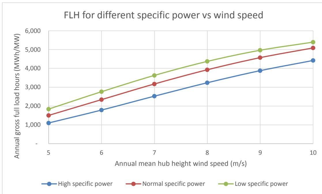
**Figure 7 Annual full load hours as a function of mean wind speed at hub height. The examples in the figure are 3 MW with 90m rotor diameter, specific powers are 472 W/m<sup>2</sup> called “high specific power” and 3.3 MW turbines with 112 m and 126 m rotor diameters, specific powers are 335 W/m<sup>2</sup> called “medium specific power” and 265 W/m<sup>2</sup> called “low specific power”.**
