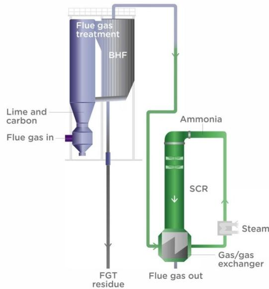
**Figure 4 Flue gas treatment system (dry/semi-dry) including reactor with injection of hydrated lime, a bag house filter and an SCR system with gas/gas heat exchanger, steam reheater, ammonia injection and catalyst.**
