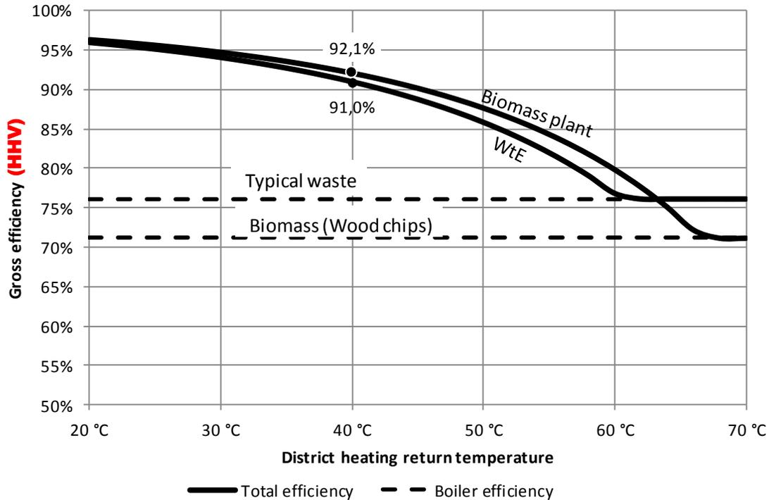
Figure 7. Total HHV-based efficiency estimate for WtE plants<sup>7</sup> and biomass plants<sup>8</sup> given varying DH return temperatures [5] – or temperature of the cold media of a heat pump.
