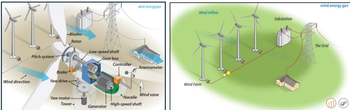
Figure 2 General turbine technology and electrical system.
