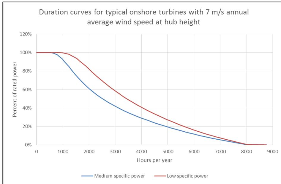
**Figure 4** Duration curve for typical modern onshore wind turbines (> 2 MW) located in Denmark (DTU International Energy Report - Wind Energy, 2014). The two curves are based on the V117 3.3 MW (307 W/m<sup>2</sup>) and V126 3.3 MW (265 W/m<sup>2</sup>) wind turbines.
