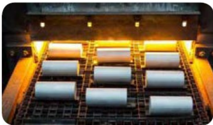
Figure 4: Queen City Forging - heating billets, from [1]
