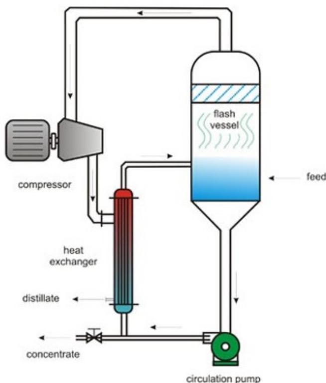
**Figure 1: Simplified illustration of the MVR cycle. For a water treatment system, the feed is dirty water, the concentrate is highly concentrated pollutants, and the condensate/distillate is pure water.**
