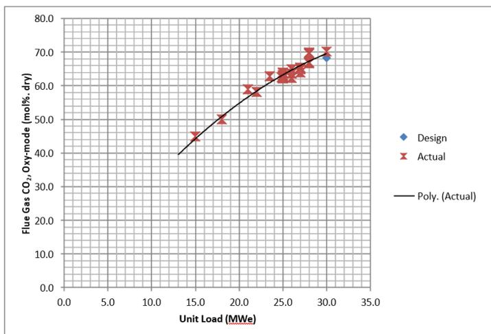
Figure iii-6 CO<sub>2</sub> concentration dependent on load at Callide oxy-fuel plant from [52].
