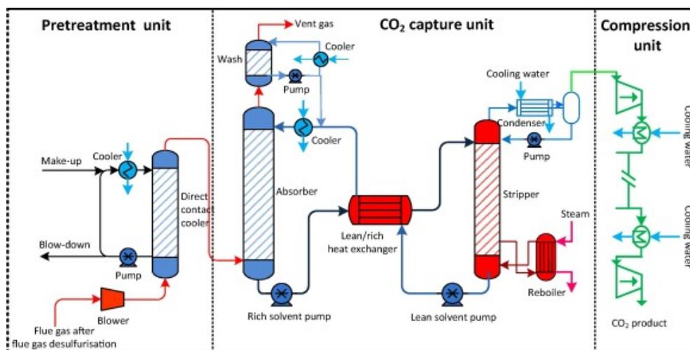
**Figure ii-1.** Schematic illustration of amine based CO<sub>2</sub> capture process as reported in [11]. Flue gas is cooled in a pre-treatment unit prior to entering the CO<sub>2</sub> capture unit where CO<sub>2</sub> is washed out by an amine solution. The CO<sub>2</sub> gas is stripped of the amine solution whereby it is regenerated by applying heat in a stripper (desorber). The recovered CO<sub>2</sub> may be compressed and dehydrated for transportation.
