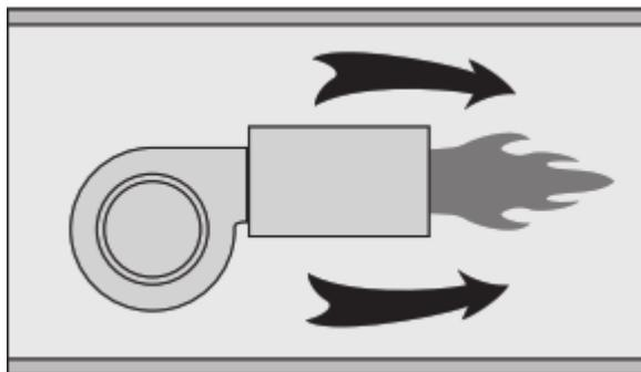
Figure 1: A burner in a duct [10].
