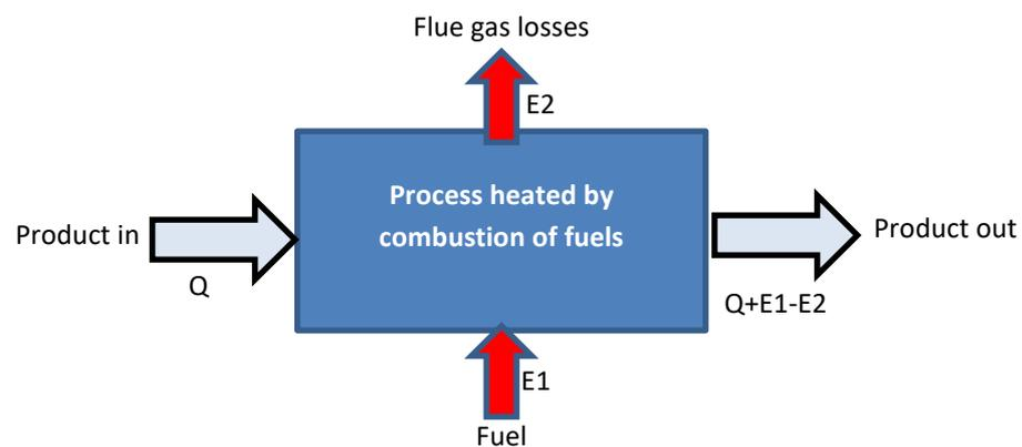
Figure 5: Energy balance of a direct firing process.
