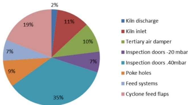
Figure iii-4 Overview of air-leakages at a typical Portland cement plant. [38]
