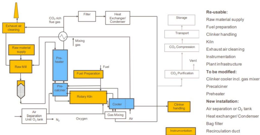
Figure iii-3 General Scheme for an oxy-fuel retrofit concept: White: To be installed new, Blue: To be utilized from existing plant, Yellow: To be modified, Grey: Not needed for proof of concept. [48]
