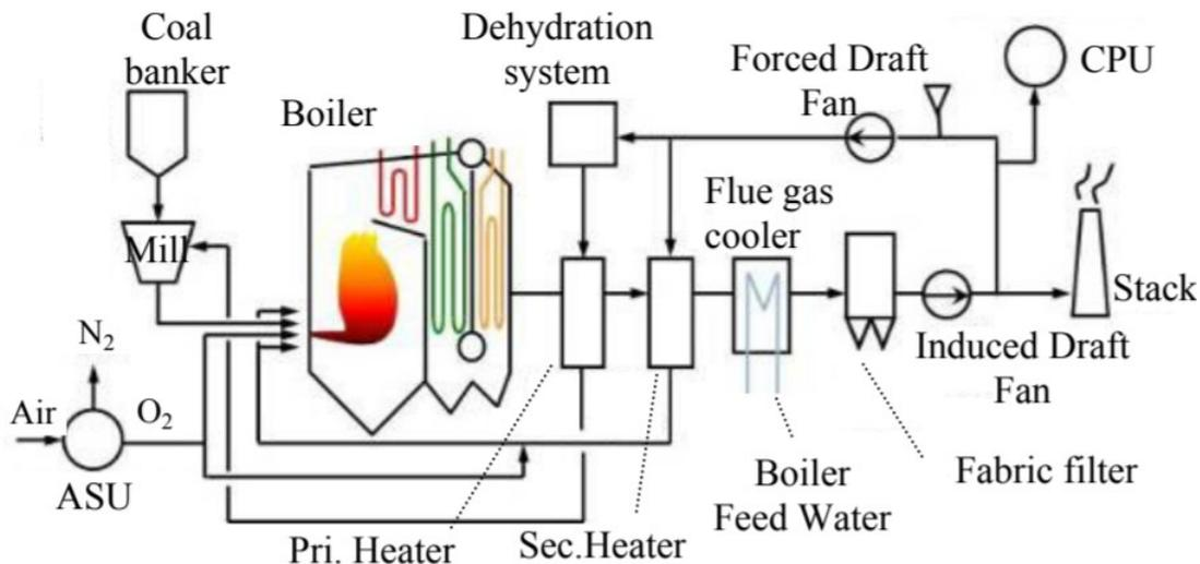
Figure iii-9 Illustration of the rebuilds needed to retrofit Callide A unit 4.[52]
