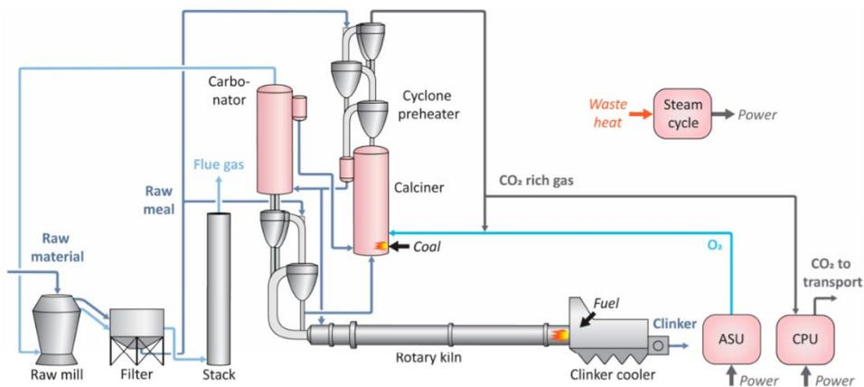
Figure iii-5. Partial oxy-fuel combustion with integrated Calcium looping (49)
