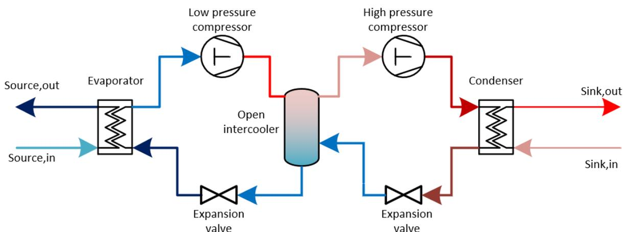
Figure 1: Sketch of two-stage compression heat pump
