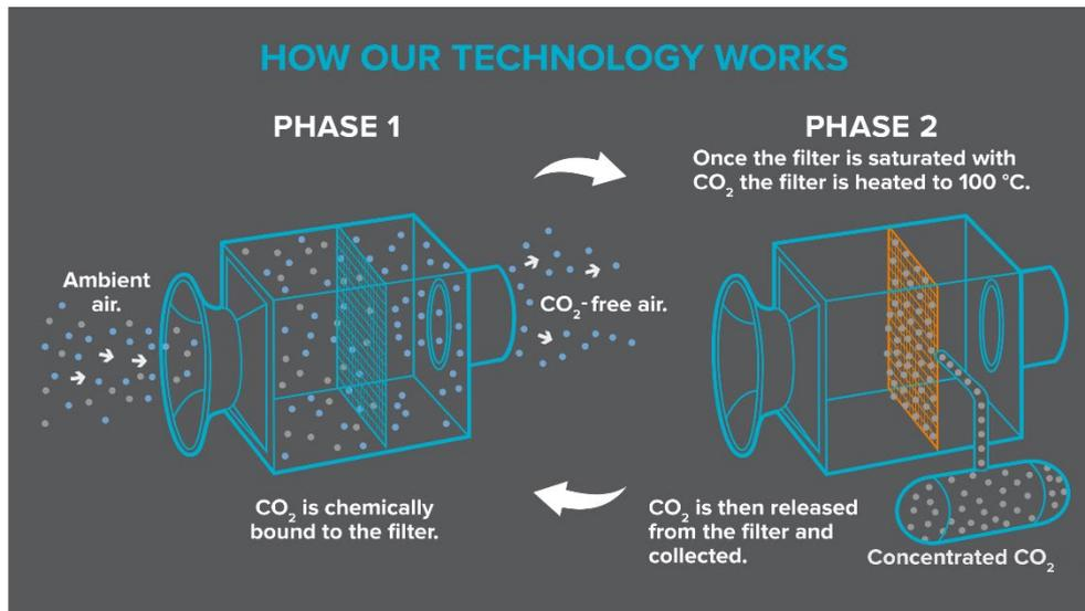
Figure iv-1. Illustration of working principle of Climeworks low temperature adsorption DAC process. Source: [www.climeworks.com](http://www.climeworks.com)
