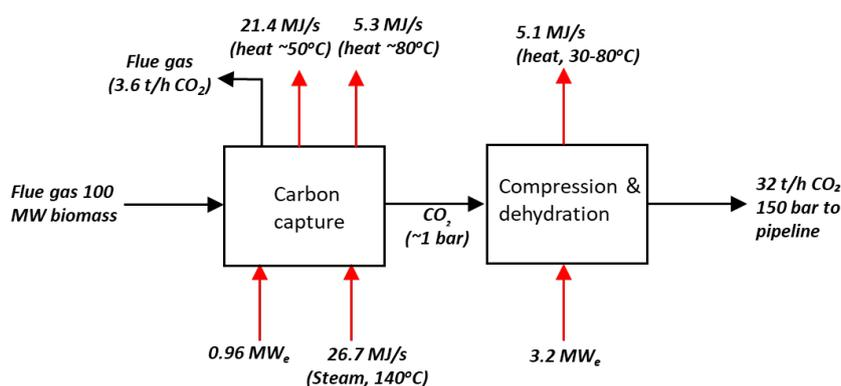
**Figure ii-2. Illustration of energy balance for a CO<sub>2</sub> capture and compression plant treating all flue gas from a 100 MW<sub>th</sub> biomass boiler that is equipped with flue gas condensation. 90% of the CO<sub>2</sub> in the flue gas is captured corresponding to 32 t CO<sub>2</sub> output per hour. Black arrows: Mass streams. Red arrows: Energy streams.**
