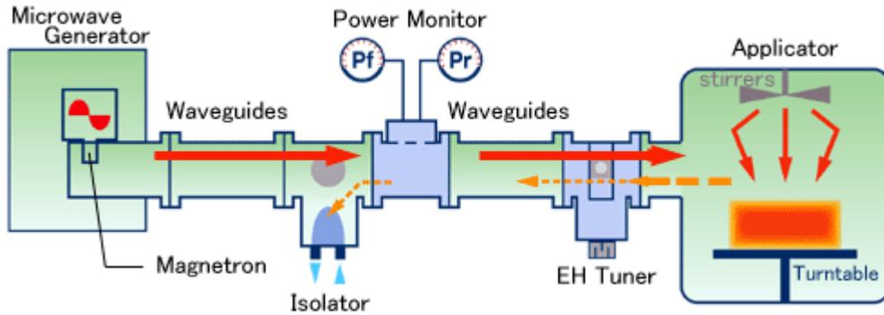
Figure 1: Schematic drawing of microwave system [7]
