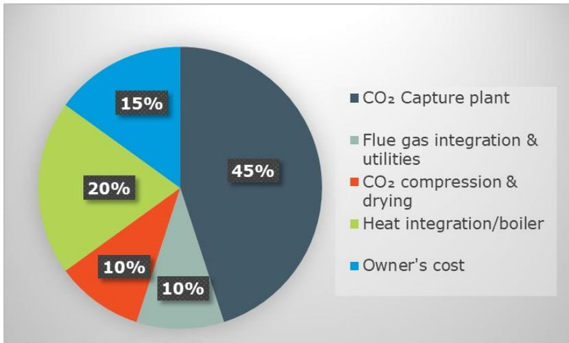
Figure ii-7. Estimated CAPEX distribution of a complete CC plant retrofit installation based on data from [28].
