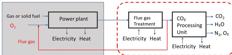
**Figure 7: Oxy-fuel combustion**
