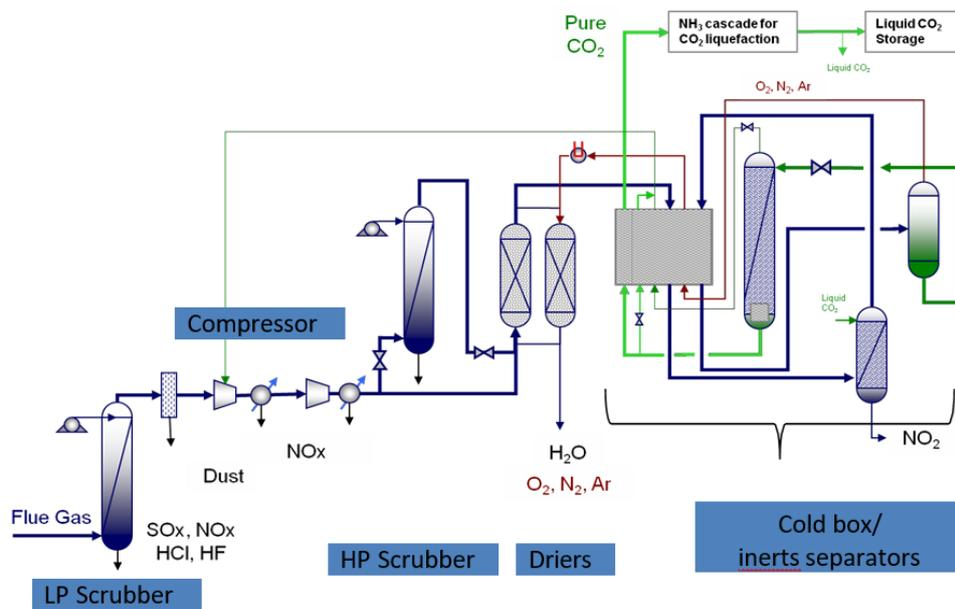
Figure iii-7 Upgrading of raw CO<sub>2</sub> at Callide oxy-fuel CCS. [44]
