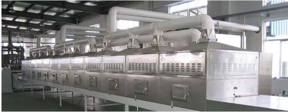
Figure 3. Industrial microwave heating system (Max Industrial Microwave)
