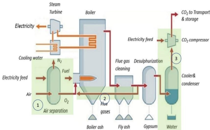
Figure iii-1 Schematic illustration of oxy-fuel combustion (25).
