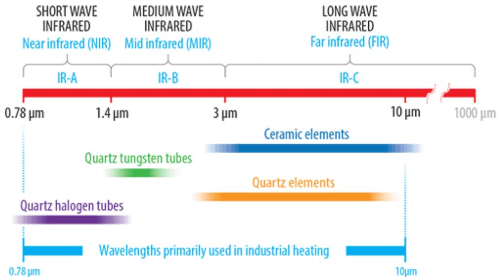
**Figure 2: Infrared subdivisions and types of infrared element for different wave length**
