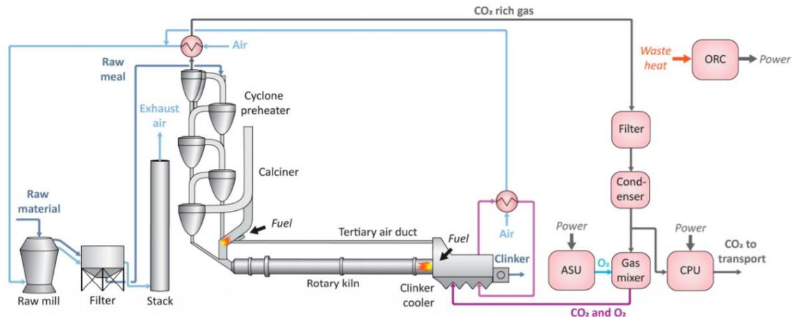
Conversion to oxy-fuel firing might seem uncomplicated, however the cement kiln process itself must be modified. The gas atmosphere in the clinker cooler, the rotary kiln, the calciner and the preheater is changed, and some of the flue gas is recycled.
