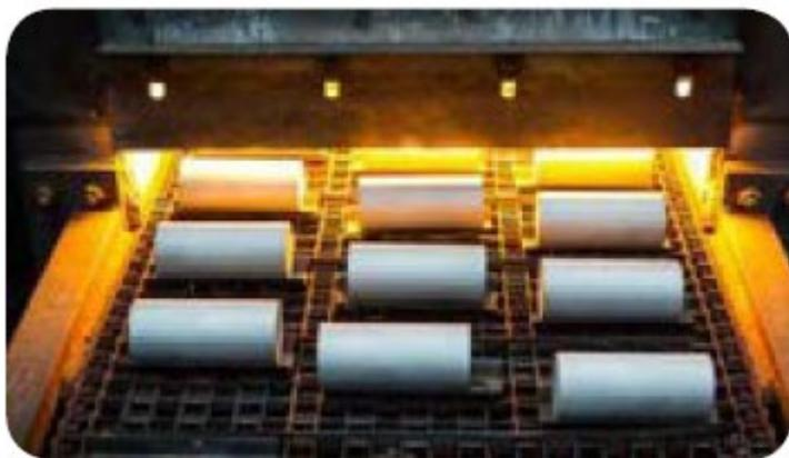
Figure 4: Queen City Forging - heating billets, from [1]
