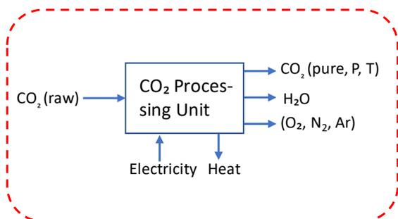
Figure 9. Illustration of CO<sub>2</sub> processing (conditioning) unit.
