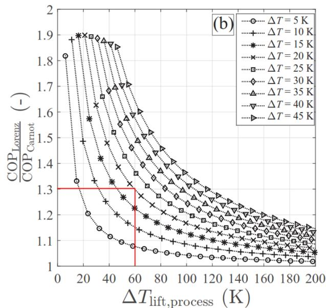
Figure 2: Theoretical advantage of using a HACHP compared to a normal vapour compression heat pump, as a function of temperature lift (x-axis), and glide [4].  $\Delta T_{Lift,process} = \text{Sink outlet} - \text{Source inlet}$
