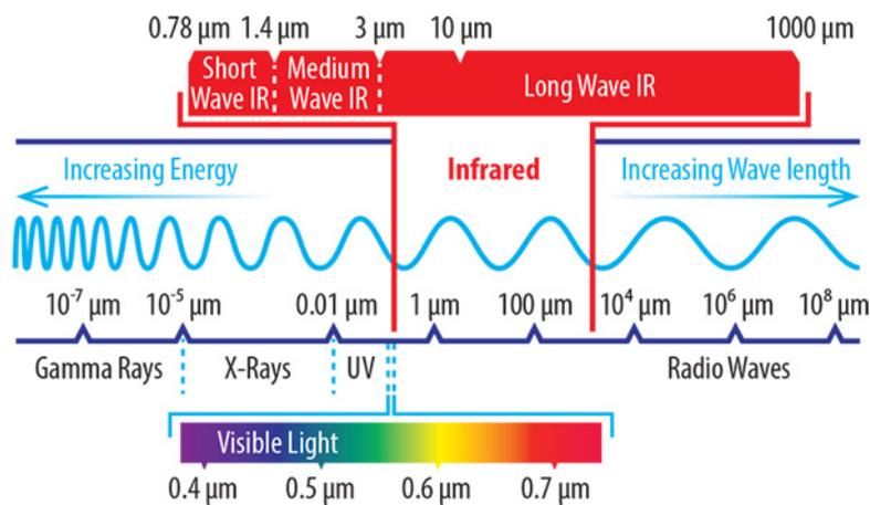
Figure 1: Infrared in the electromagnetic spectrum [2]
