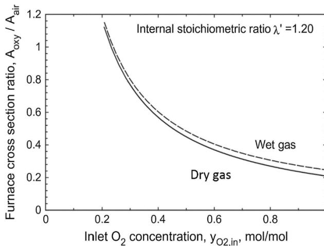
Figure iii-8 Potential to reduce boiler size by increasing  $\text{O}_2$  concentration. [45]
