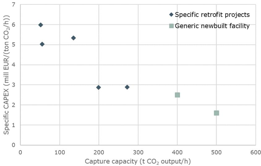
Figure ii-6. Specific CAPEX cost of complete CC plant installations including CO<sub>2</sub> compression, integration and utility costs vs. CC plant capacity (data from Table ii-4).
