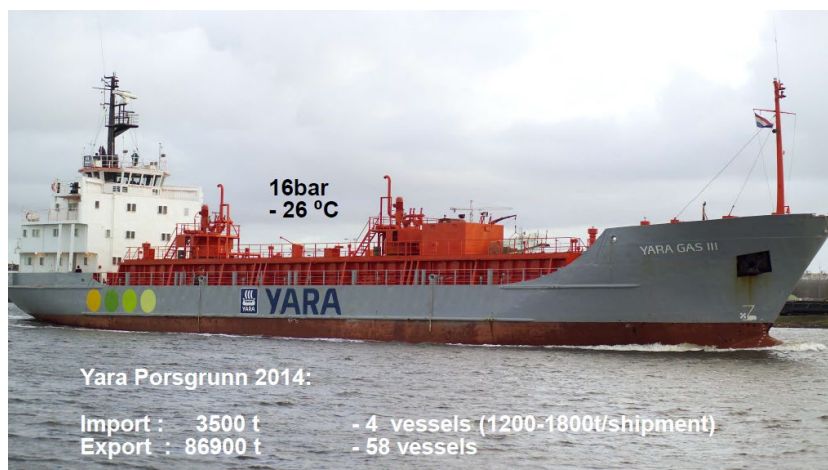
Figure 6. M/T Yara Gas III liquid CO 2 carrier. [7]
