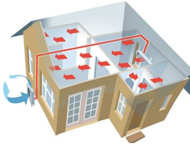
Figure 34 Illustration of a heating system based on a ventilation heat pump.
