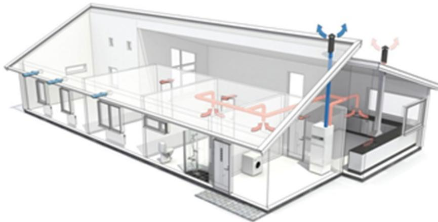
Figure 35 Illustration of a heating system based on a ventilation heat pump.
