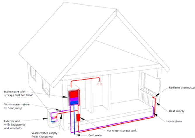
**Figure 32 Illustration of a heating system based on an air-to-water heat pump (monobloc).**
