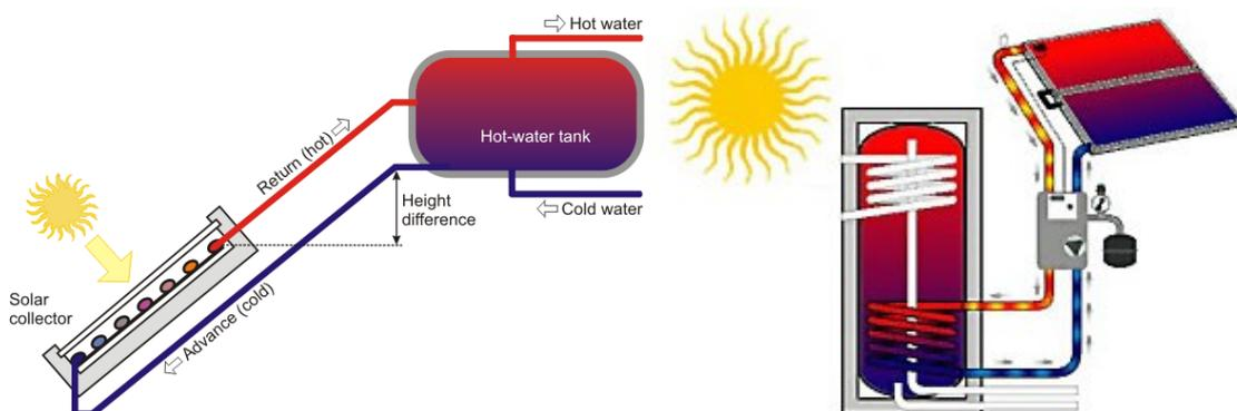
**Figure 45: Small solar heating system for domestic hot water. To the left a pumped system where auxiliary heat is supplied to the upper heat exchanger coil. To the right a thermosyphon system without pump. In such a system the circulation of the heat transfer fluid is driven by natural convection rather than a mechanical pump. By far the most systems are equipped with a pump.**
