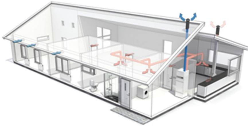
Figure 35 Illustration of a heating system based on a ventilation heat pump.
