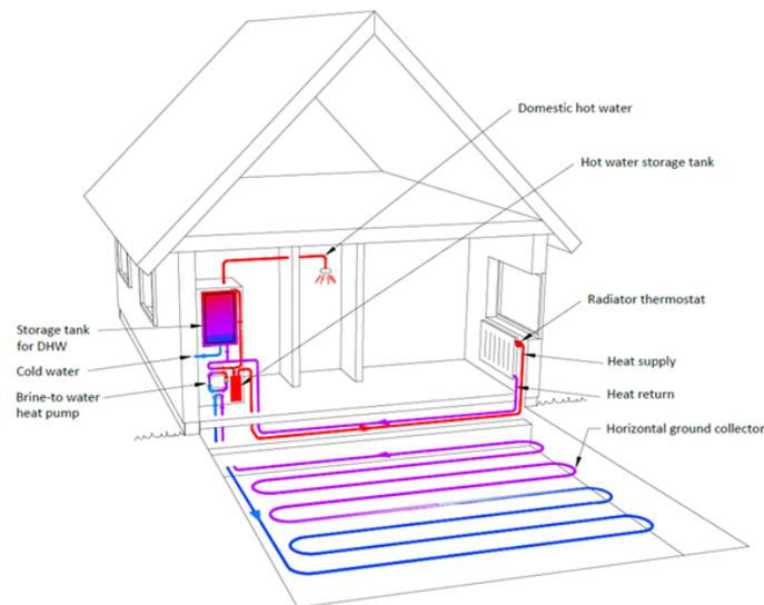
**Figure 33 Illustration of a heating system based on a ground source heat pump (horizontal collector).**
