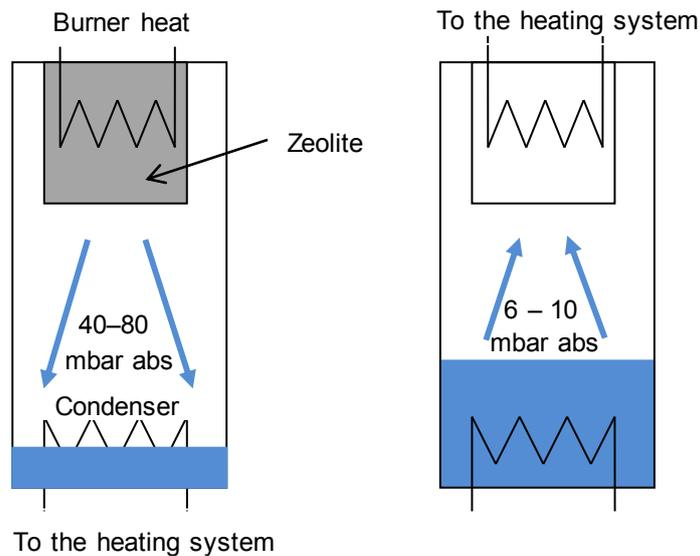
Figure 1 Sketch of the basic adsorption process [16], Residential gas-fired sorption heat pumps. Test and technology evaluation, DGC 2008
