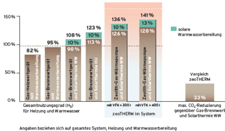
Figure 3 Vaillant Zeolite adsorption heat pump efficiency (based on lower calorific value) [11]
