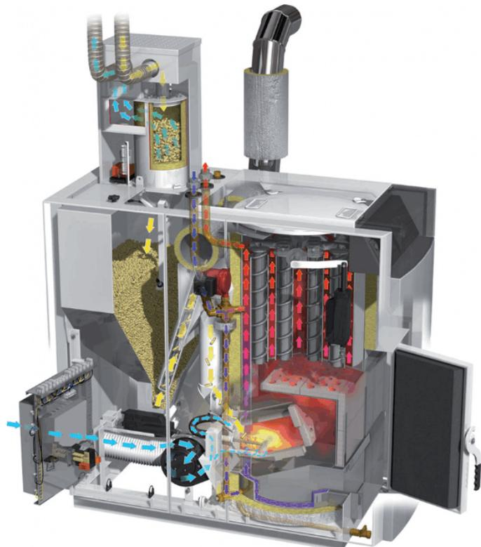
Figure 12: Biomass boiler, automatic stoking
