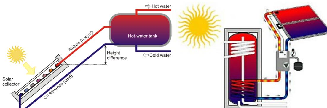
**Figure 15: Small solar heating system for domestic hot water. To the left a pumped system where auxiliary heat is supplied to the upper heat exchanger coil. To the right a thermosyphon system without pump. In such a system the circulation of the heat transfer fluid is driven by natural convection rather than a mechanical pump.**
