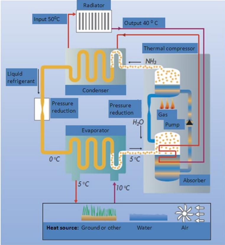
Figure 1 Operating principle for gas absorption heat pump [10]
