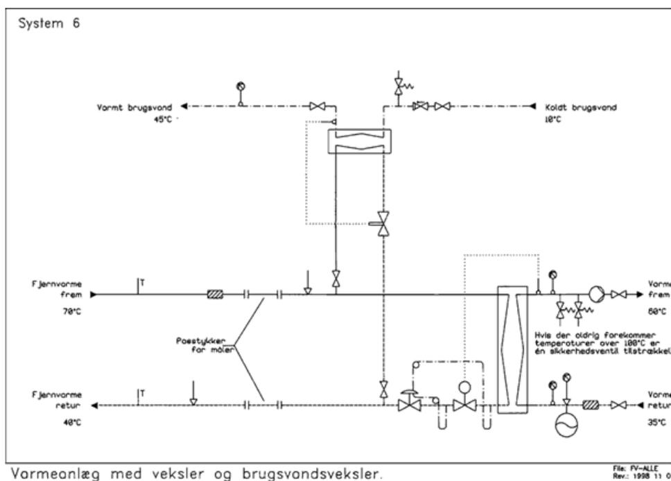
**Figure 7:** Indirect district heating substation with domestic hot water heater and heat exchanger for space heating in a one-family house. A branch pipe is connecting the building with the district heating network [1].
