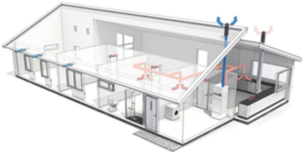
**Figure 5: Ventilation air heat pump**
