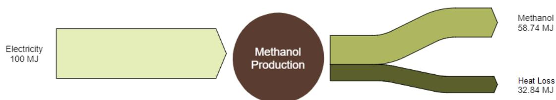
Figure 2 Methanol from Power Energy Balance
