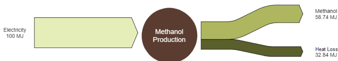
Figure 2 Methanol from Power Energy Balance
