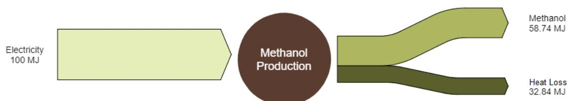
Figure 2 Methanol from Power Energy Balance
