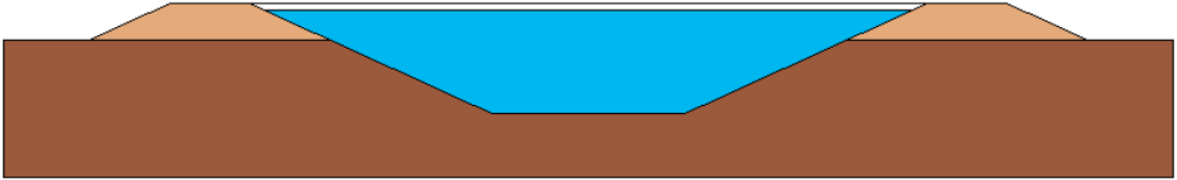
Figure 2: Principle sketch of a pit heat storage cross section [15].
