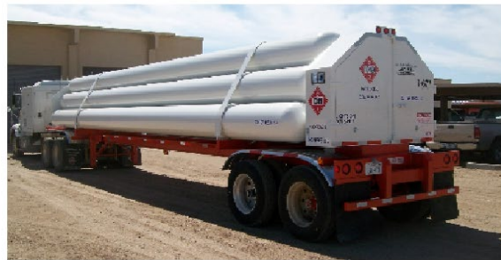
Hydrogen tube truck/trailer
