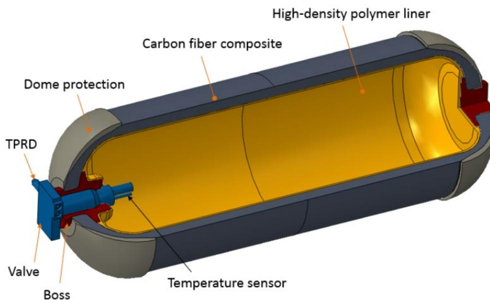
TPRD = Thermally Activated Pressure Relief Device
