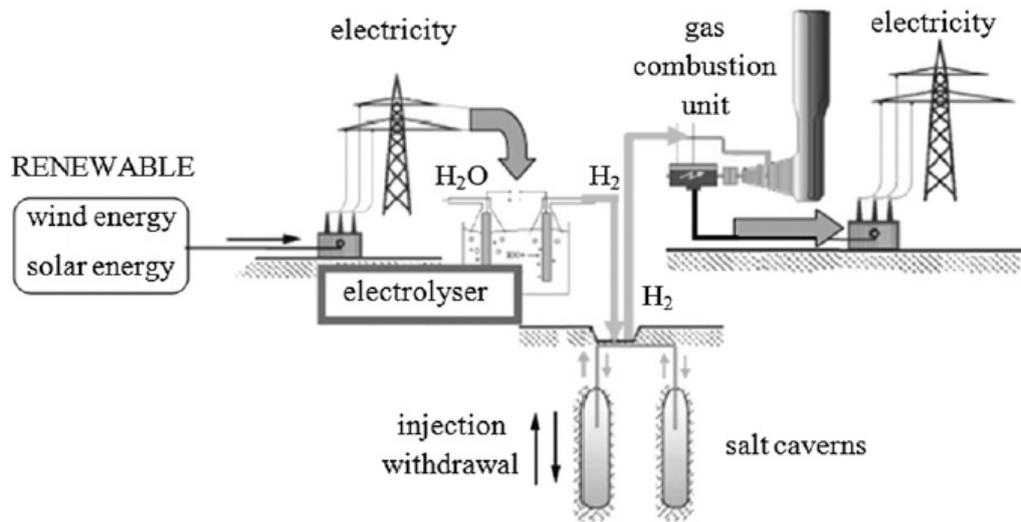
Figure 15: An illustration of H<sub>2</sub> storage in salt caverns. As an example it is shown that the hydrogen can be used for power generation. [56]
