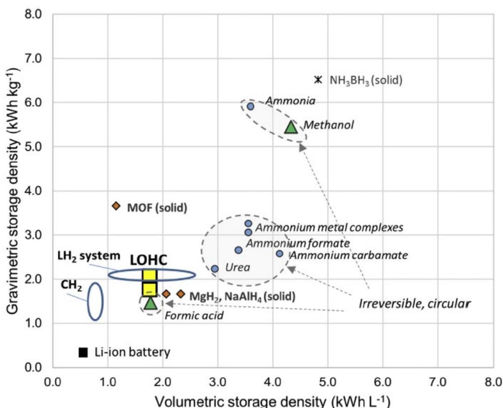
Figure 11: Properties of different hydrogen storage technologies [45]
