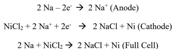
During charge the reverse reaction occurs. The reaction has a full cell potential of 2.58 V at 300 °C. The operating temperature is 250 °C to 350 °C to ensure sufficient Na ionic conductivity through the BASE [4]. A lower limit operation temperature of 150 °C is required to maintain liquid NaAlCl<sub>4</sub> [1]. An illustration of the charging reaction can be seen in Figure 3.
