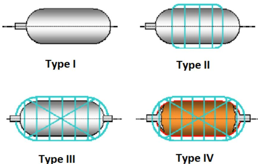
Figure 6: Schematic of different hydrogen pressure tank types[18]
