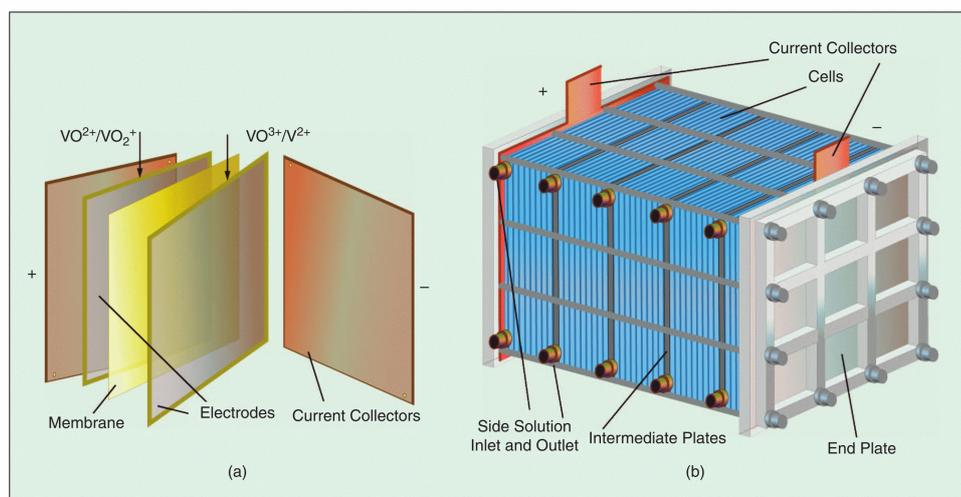
Figure 2: a) Reaction cell. b) Typical stack [2].
