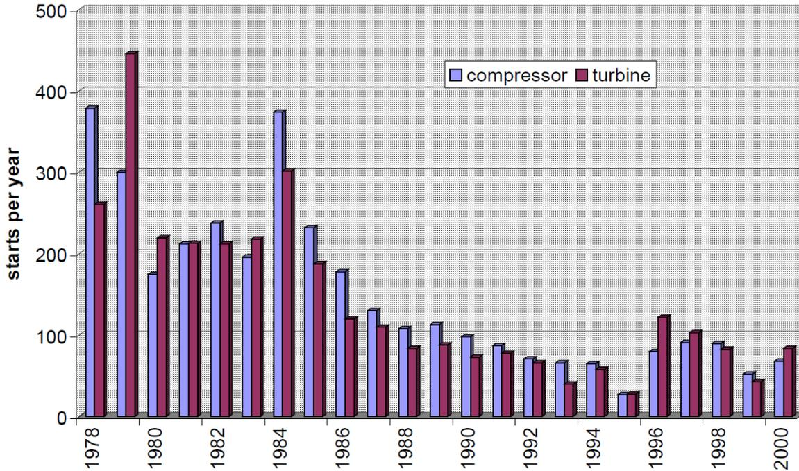
Figure 5: Number of compressor starts (charges) and turbine starts (discharges) for the Huntorf facility for the period between 1978 and 2000 [10]
