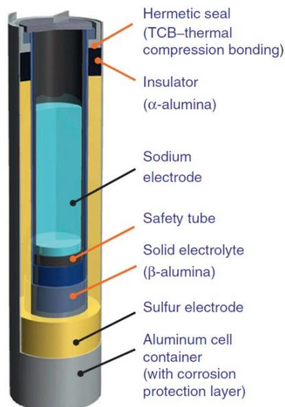
Figure 1: Schematic of a Na-S battery cell. [4]
