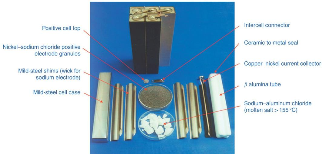
Figure 2: Na-NiCl<sub>2</sub> battery cell components [1].
