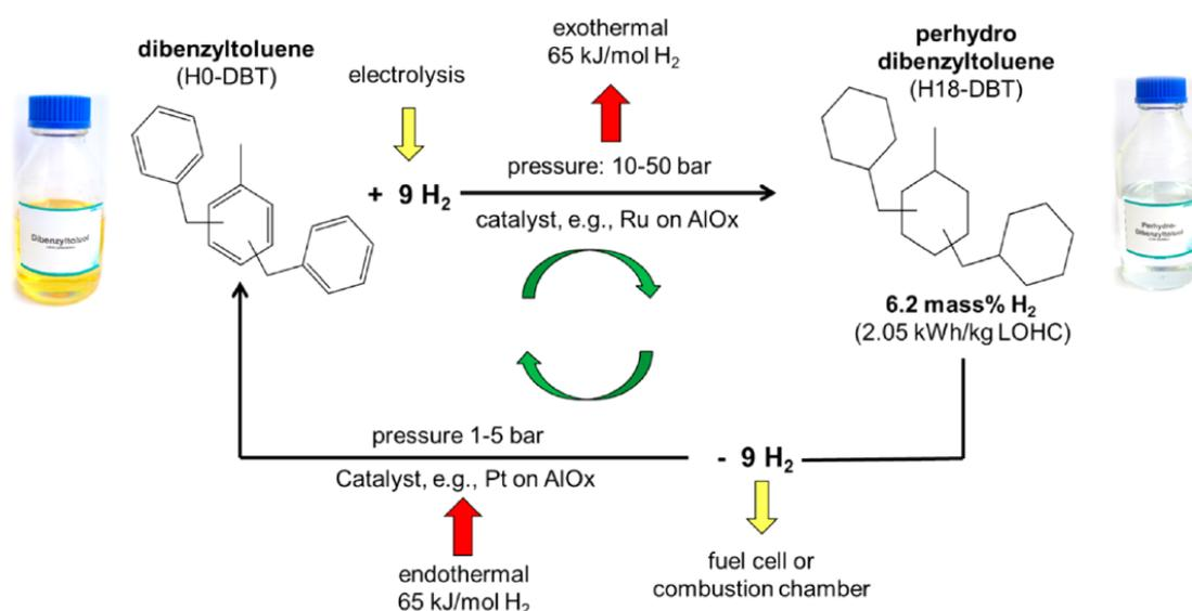
Figure 13: Hydrogen storage using DBT-LOHC system[50]
