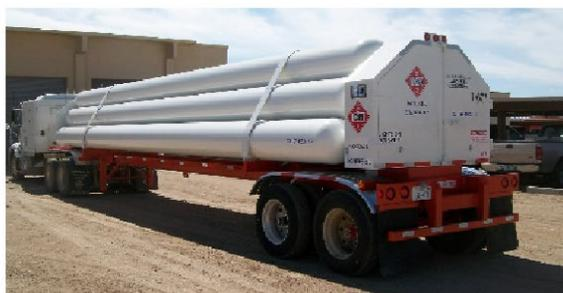
Hydrogen tube truck/trailer
