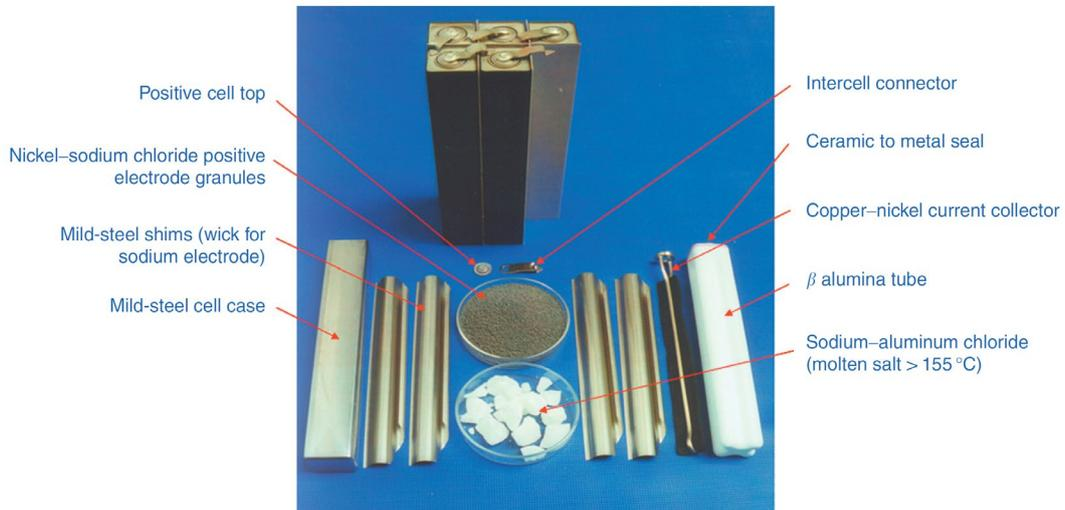
Figure 2: Na-NiCl<sub>2</sub> battery cell components [1].
