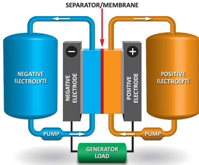
Figure 1: Schematic of flow battery [1].
