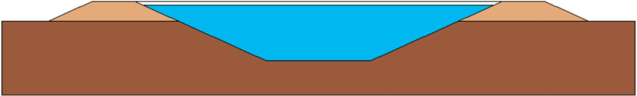
Figure 2: Principle sketch of a pit heat storage cross section [15].
